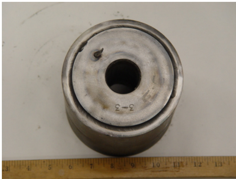
Fig. 4.6. Back side of bimetalllic steel billet with welds, weld plate, and crimped-off degassing tube.
