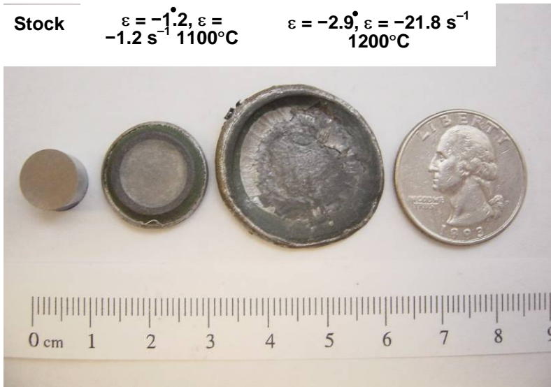
Fig. 4.54. Gleeble samples for deformation simulation. From left to right, stock material (half of pair), low extrusion ratio simulation, high extrusion ratio simulation.
