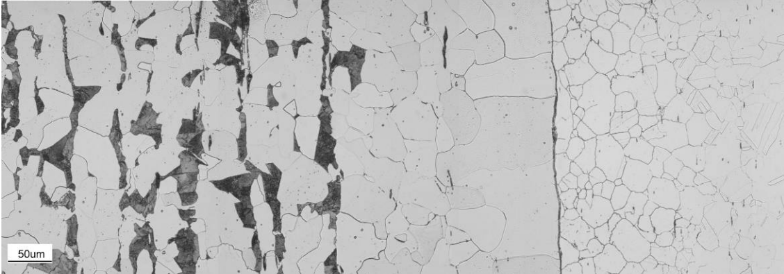
Fig. 4.52. Composite micrograph of the regions adjacent to the interface after extrusion with high extrusion ratio. The effective strain (2.9) and strain rate ( 22 \text{ s}^{-1} ) were calculated using DEFORM of (left) 1020 steel and (right) 304 stainless steel. The sample was etched with agitated 60 mL HCl, 60 mL \text{HNO}_3 , and 60 mL distilled \text{H}_2\text{O} for 30 s.
