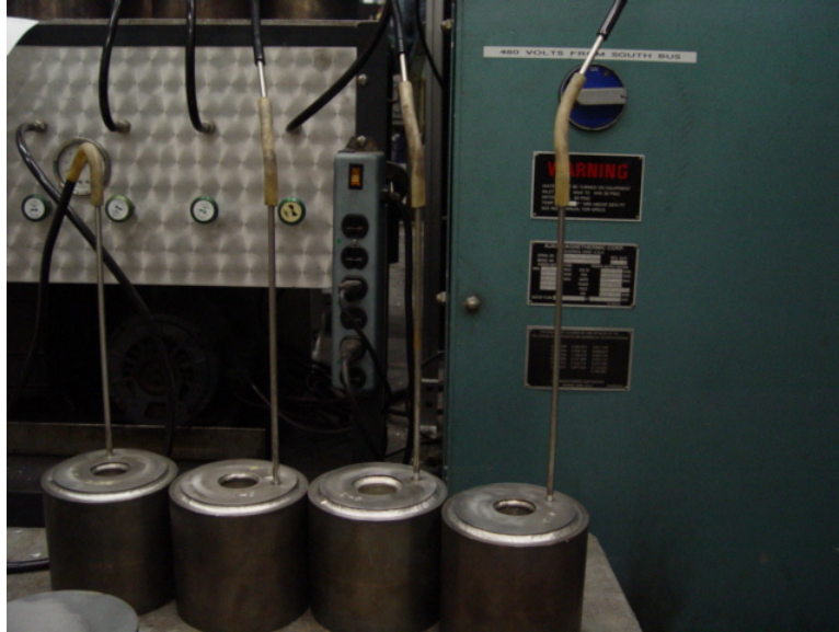
Fig. 4.5. Bimetalllic billets being degassed.
