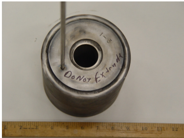
Fig. 4.4. Back side of bimetallic steel billet with welds, weld plate, and degassing tube.
