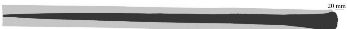
Fig. 3.8. Co-extruded rod of modeling material, hard core/soft sleeve, showing the core ballooning at the front of the extrudate (right) and core pinch-off at the back end (left).
