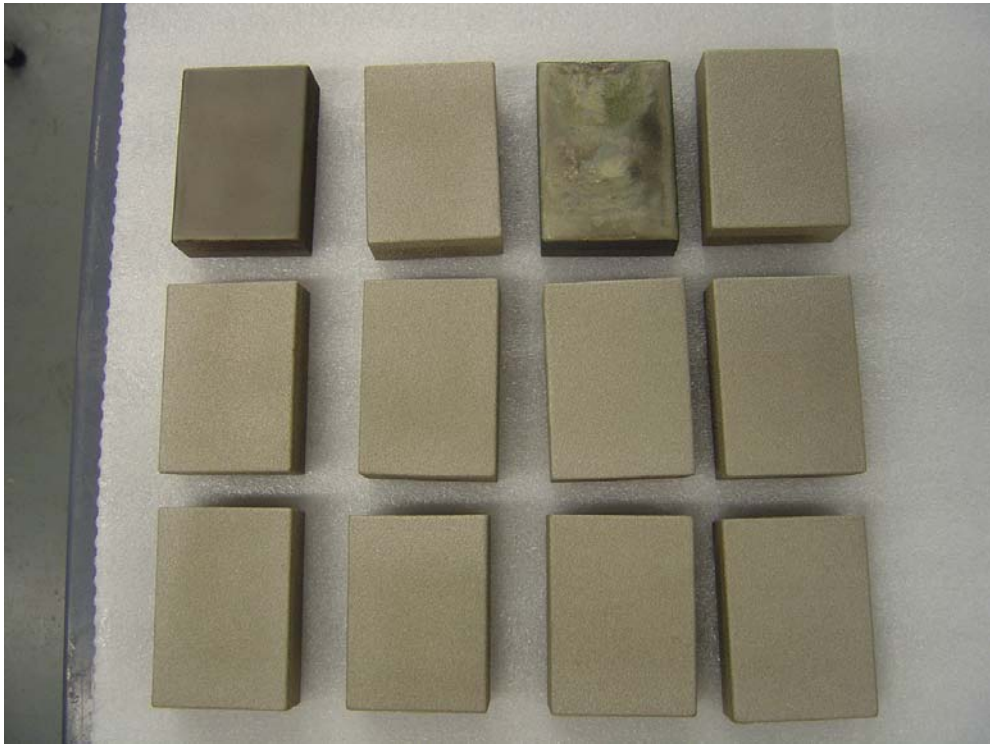
Figure 14. Wider area plasma fused coatings on steel substrate
