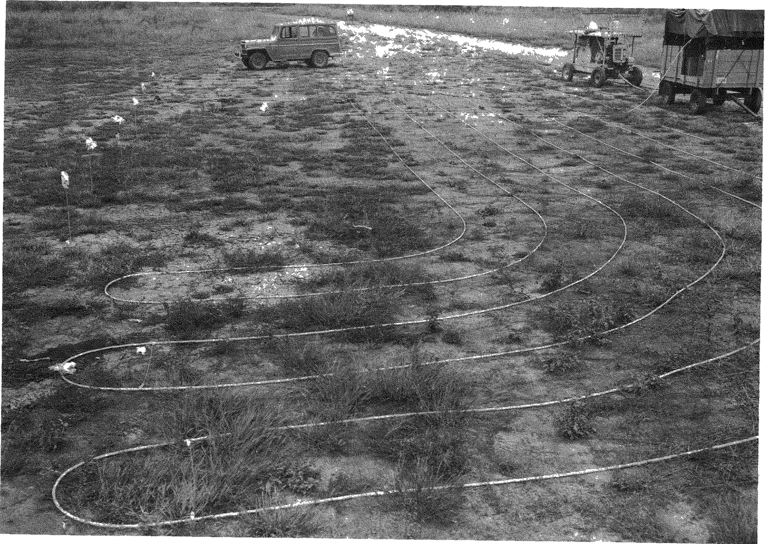
Fig. 3 2—Source tubing positioned on the ground around a “phantom” type “D” house
