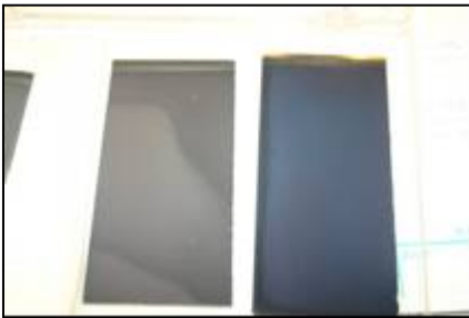
Figure 4a: Se/S treated and CdS deposited
