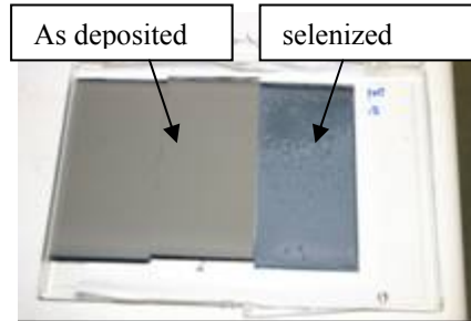
Figure 8b: As deposited and Se treated
