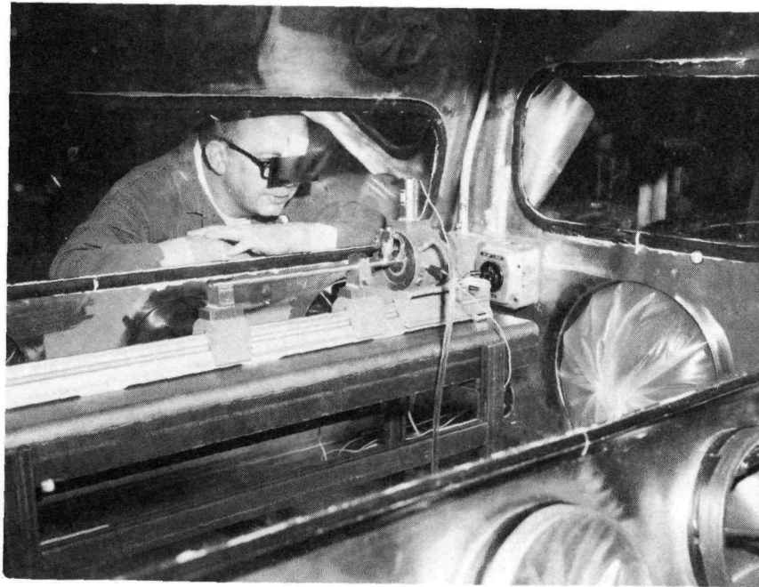
FIGURE 16. VIEW OF WELDING FIXTURE AS SET UP IN GLOVE BOX
