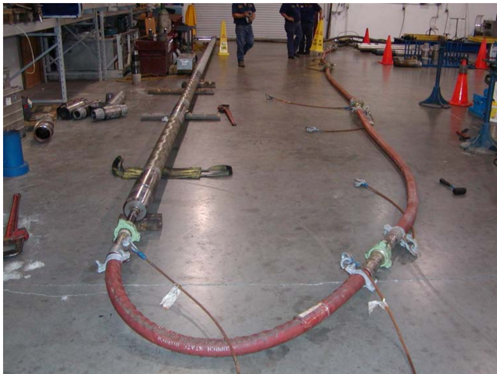
Figure 6 Composite Drill Pipes Placed Into Flow Loop
