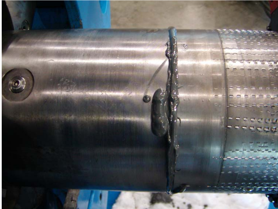
Figure 5 Torqued CDP Tool Joints
