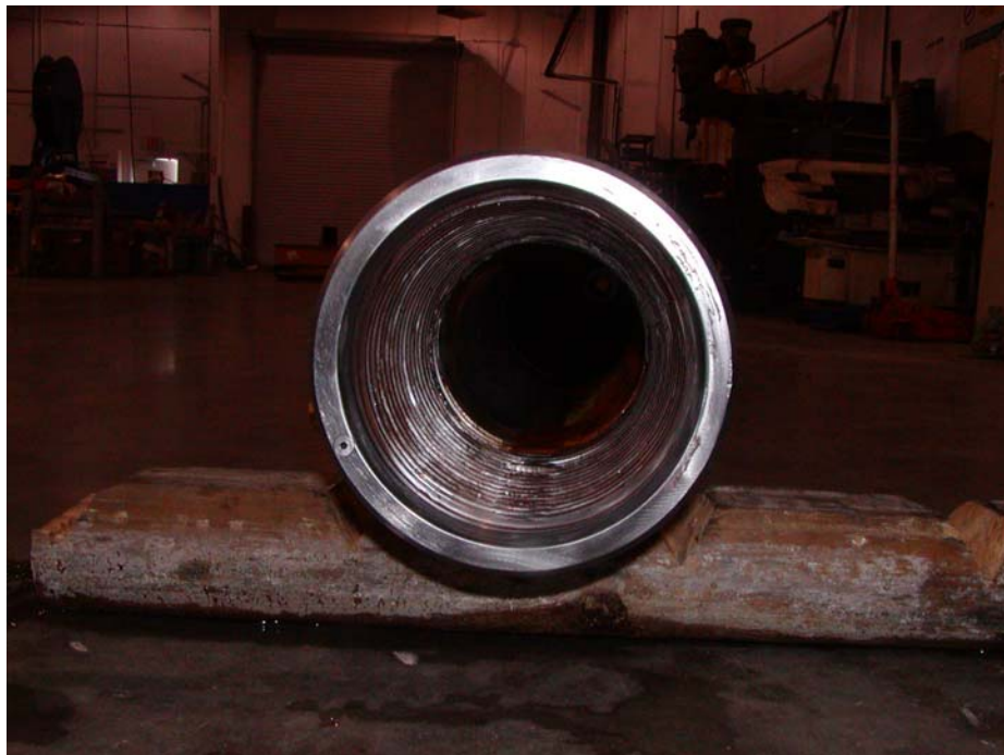
Figure 2 CDP Box Connection with Bayonet Retracted
