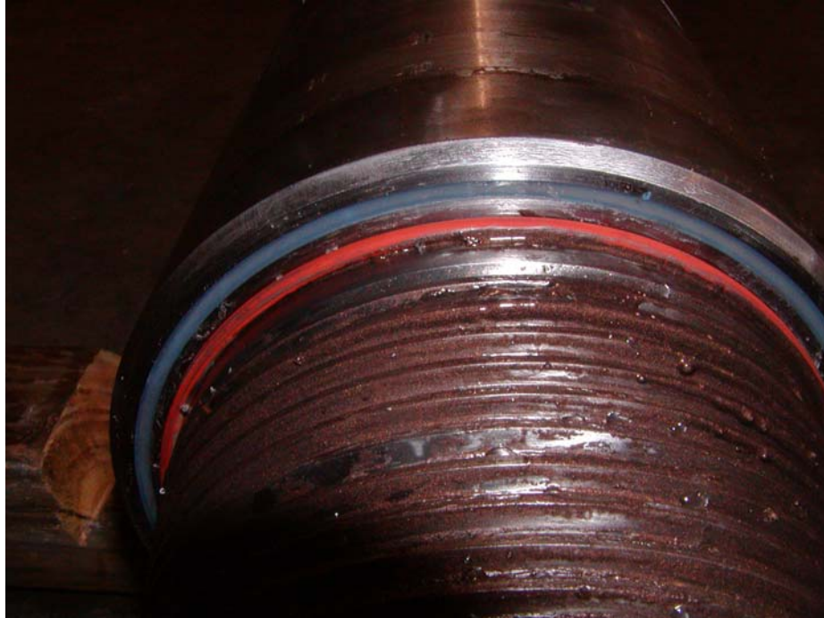
Figure 3 CDP Pin Connection
