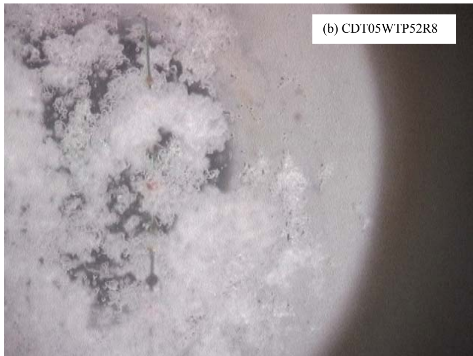
Figure 5.12 CO 2 droplet aggregation observed at (a) Q = 2.67 kg/min; T_{CO_2} = -3.25^\circ\text{C} ; T_w = 8.13^\circ\text{C} , P = 61 bar and (b) Q = 2.65 kg/min; T_{CO_2} = -2.18^\circ\text{C} ; T_w = 9.45^\circ\text{C} , P = 52 bar.
