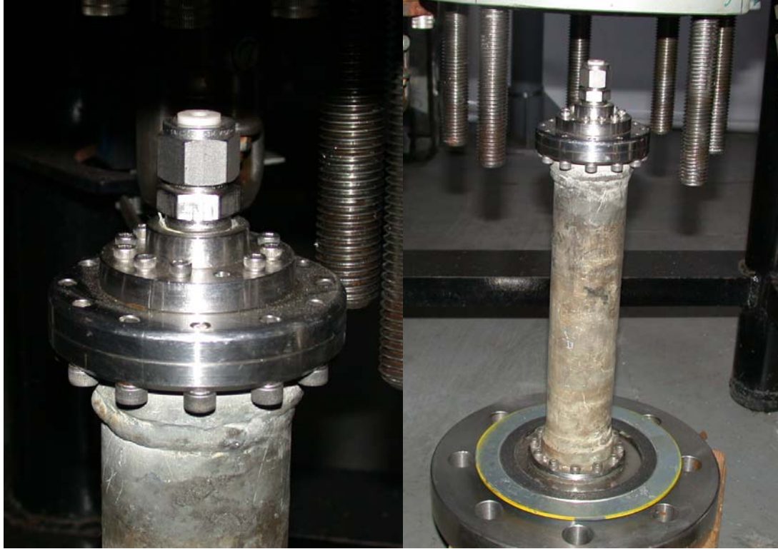
Figure 2.24 Photographs of the CO 2 injector with the 5 (T05) mm Delrin tube orifice mounted on a flange that is bolted to an opening in the bottom of the DOS.
