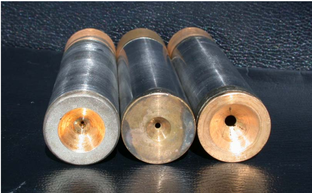
Figure 2.23 Photograph of the 1 mm (S01), 2 mm (S02) and 5 mm (S05) sharp edged orifice nozzles.
