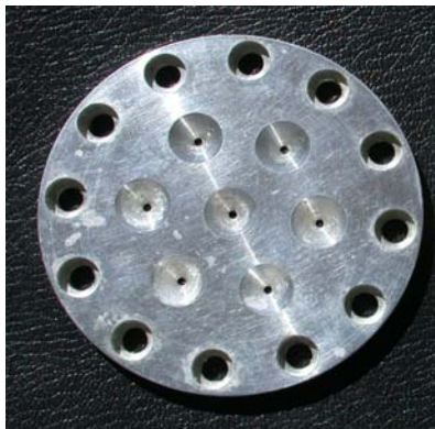
Figure 2.21 Photograph of 2 mm (C72) sharp edged, 7-orifice nozzle fabricated for the liquid CO 2 injection tests
