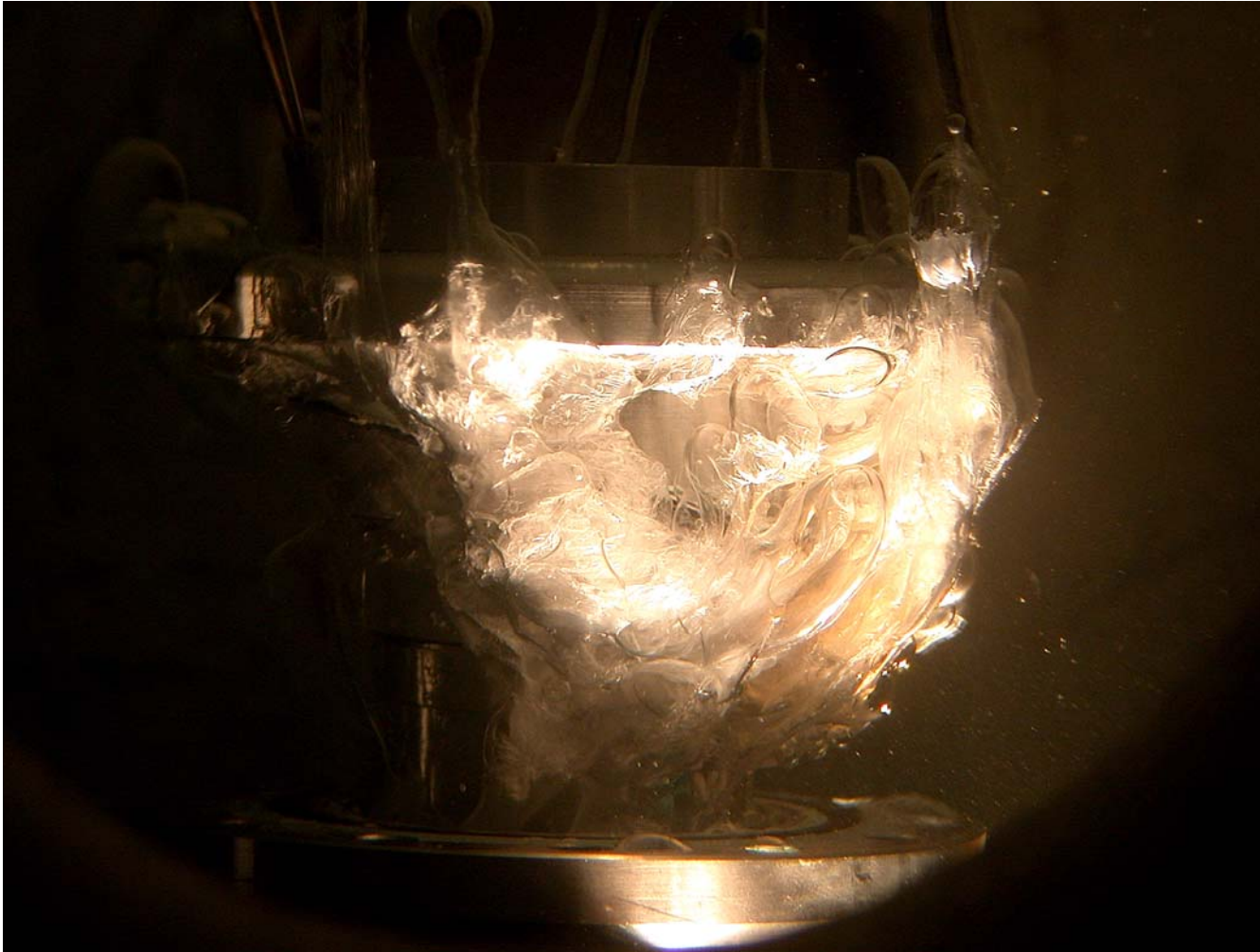
Figure 5.17 Cotton type of CO 2 hydrate observed when liquid CO 2 flows around a solid surface
