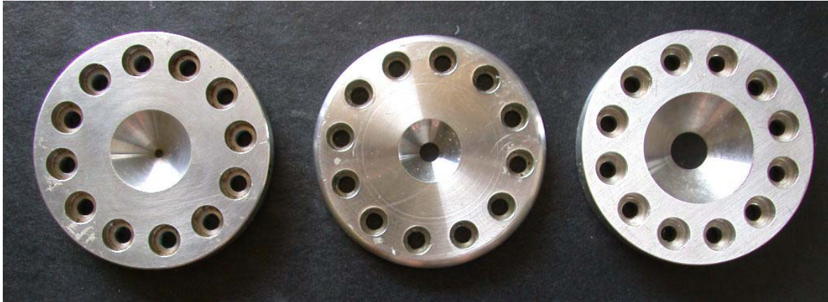
Figure 2.20 Photograph of 2 mm (C02), 5 mm (C05) and 10 mm (C10) sharp edged, single orifice nozzles fabricated for the liquid CO 2 injection tests.
