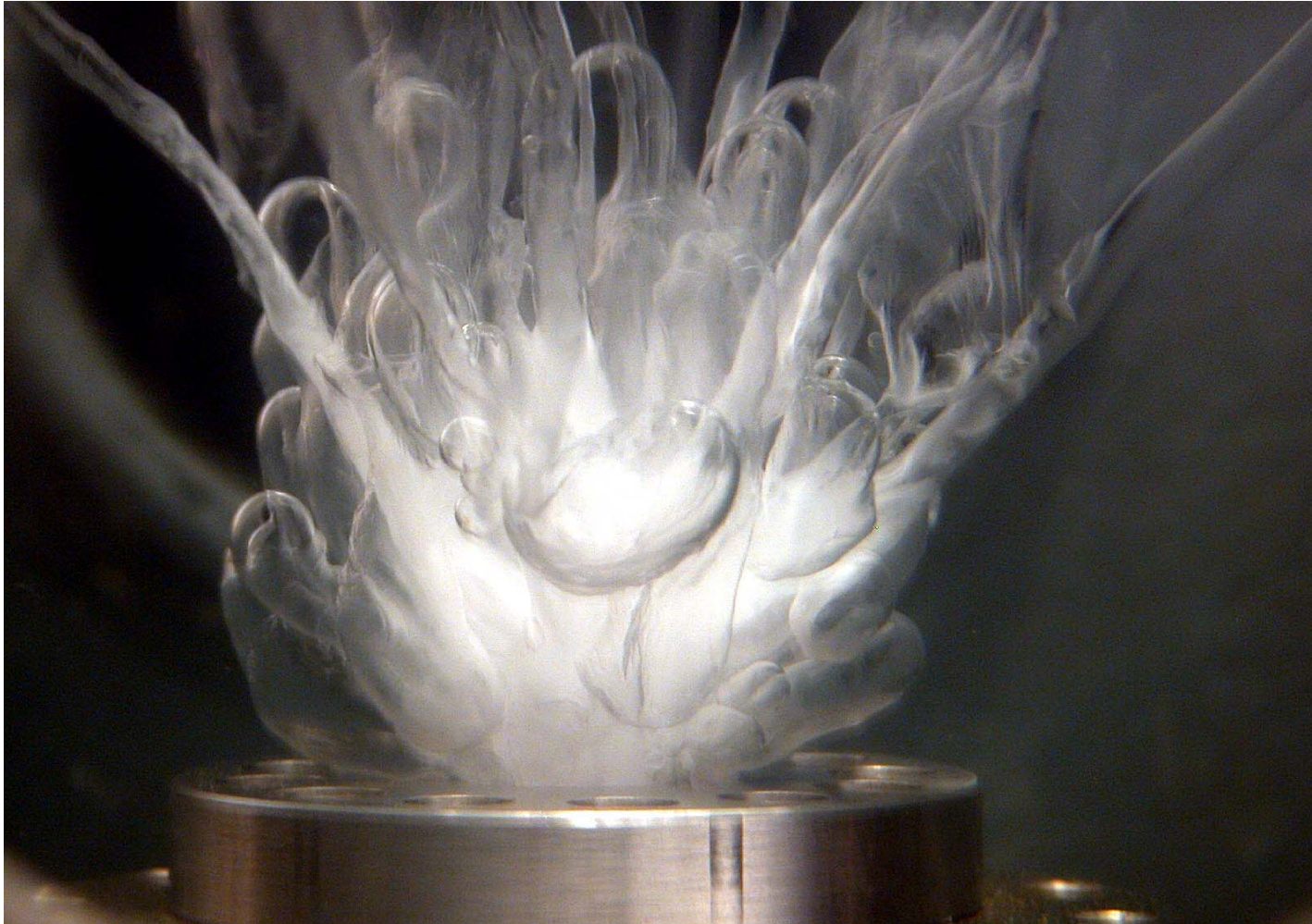
Figure 5.15 Close-up of Grape type hydrate on the top of the 2 mm sharp edge orifice (CO 2 ).
