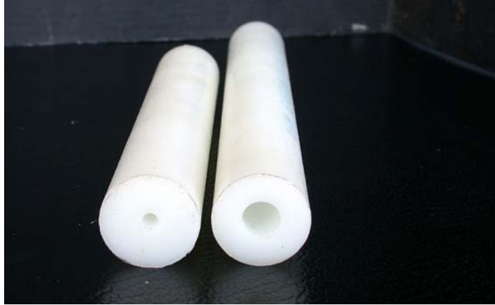
Figure 2.22 Photograph of the 2 mm (T02) and 5 mm (T05) Delrin tube orifice nozzles.
