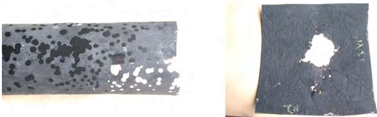
Figure 4.1. A pipe and a plate obtained from a syngas plant. Both components were attacked by metal dusting corrosion.
