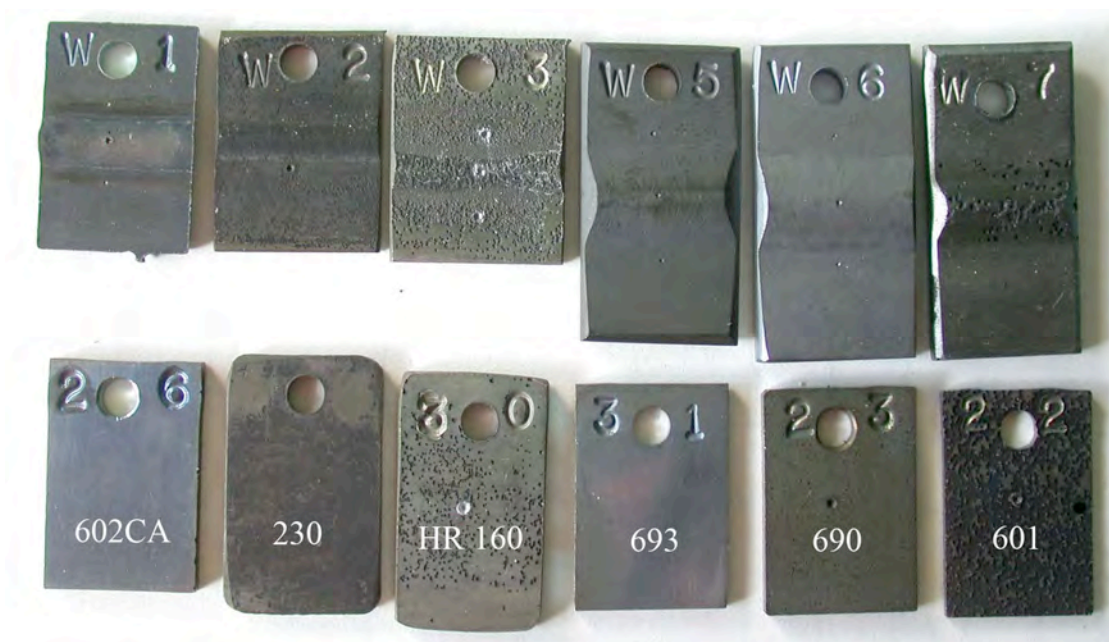
Figure 5.1. Macrophotograph of weldment and corresponding base metal specimens after 3114 h exposure at 593°C and 1 atm in a gas mixture with a carbon activity of 10^4 .
