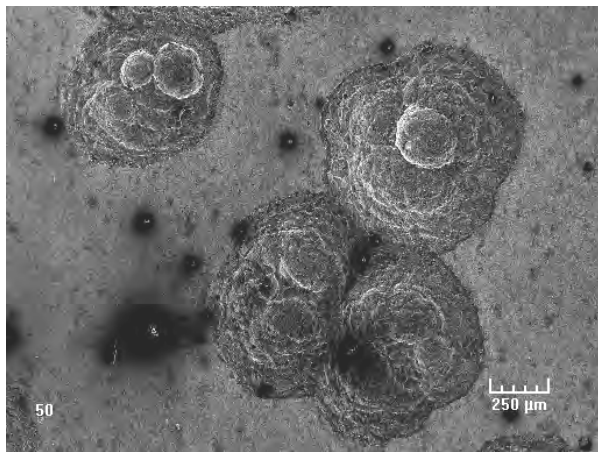
(Figure 3.5 continued.) Pit morphology as a function of time for Alloy 617 exposed to Gas 10 at 593°C and 210 psi.
