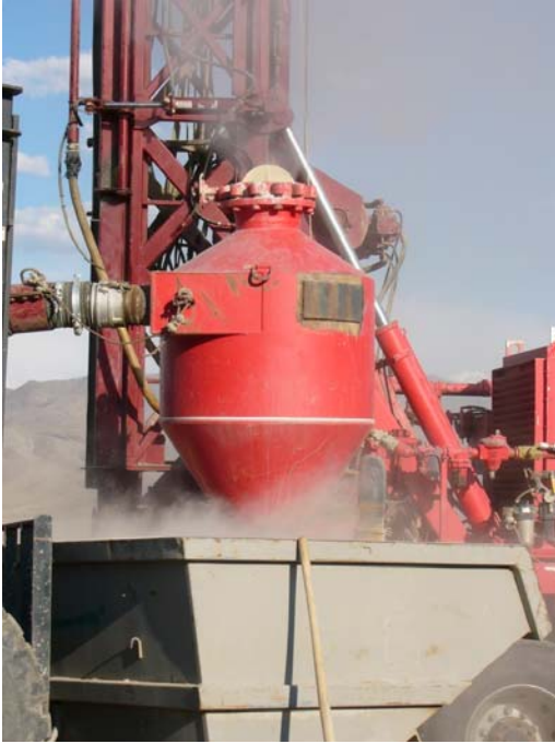
Figure 22. Compressed air carries cuttings back-up the borehole to the surface. The cyclone separator, shown on the left, slows the air velocity and allows the cuttings to be sampled, before they fall into a container.
