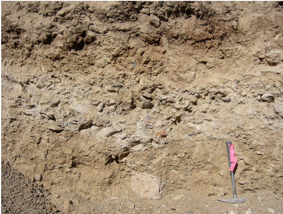
Figure 10. A poorly sorted, Quaternary gravel (a mix of a pediment gravel and alluvial deposit) on the floor of Pumpnickel Valley within the north-central portion of the project area. The section is exposed in the sump pit dug near the thermal gradient hole PVTG-3.
