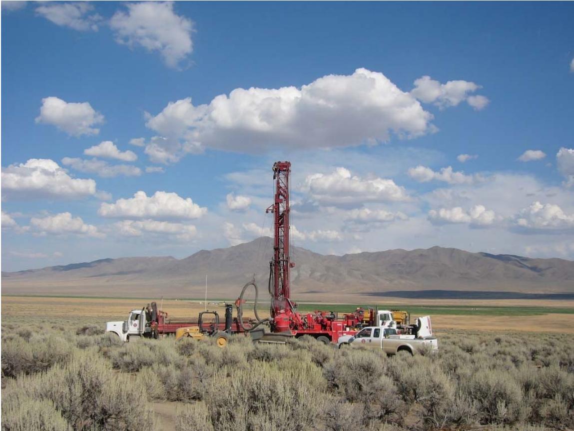
Figure 21. The GEFCO Speedstar 30K Tophead Drive air-casing advance/mud rig used by WDC of Elko, Nevada, to drill all four geothermal gradient holes in the project area. PVTG-1 site, looking ENE.
