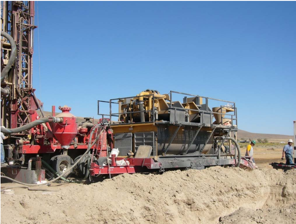
Figure 23. Vibrating screens called shale shakers allow separating the cuttings from the mud; the vibratory action of the shakers moves the cuttings down the screens (two black belts in the center of the device) where they can be sampled, and subsequently moved to the sump pit. PVTG-3 site.
