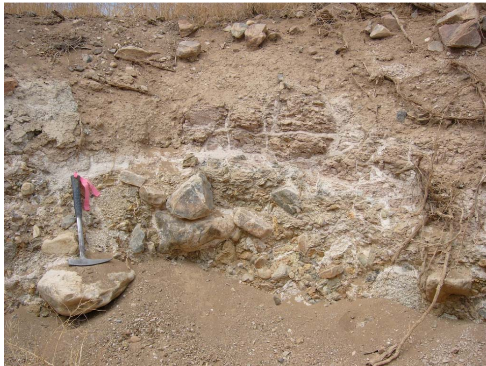
Figure 9. A typical, poorly sorted and partly consolidated, boulder-rich Tertiary gravel overlying rocks of the Preble Fm. It is exposed in a trench west of the Pumpernickel Valley fault, on the top of a hill in the section 32. A similar rock type forms lower portions of the thermal gradient holes PVTG-1 and PVTG-3.
