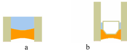
Figure 2 SealSim 1.1 currently supports the following spacer systems (a) Thermo Plastic Spacer (b) Box type spacer.
