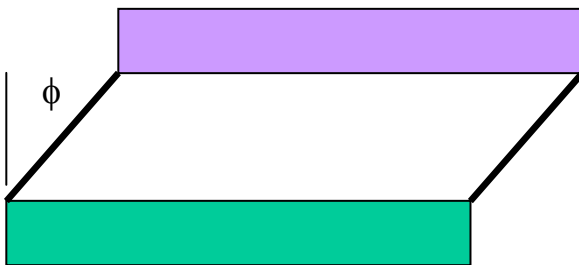
Figure 4-10. Shear stress due to bulk substrate motion
