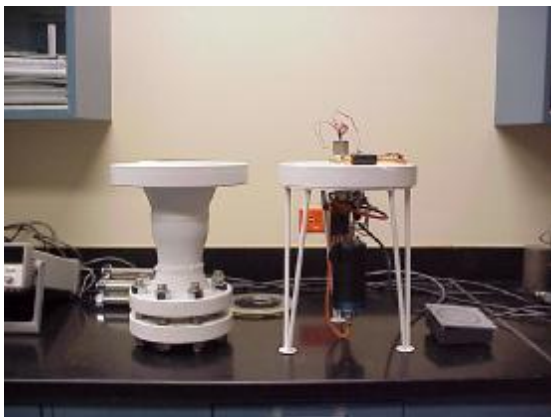
(a) Pressure vessel and CO 2 sensor.
