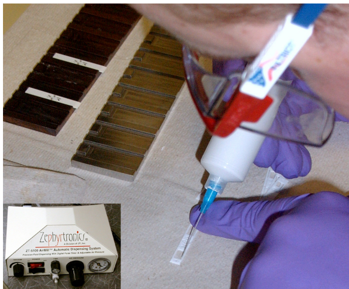
Figure 14: Application of the alumina epoxy using the Zephyrtronics Air Mill dispensing system.
