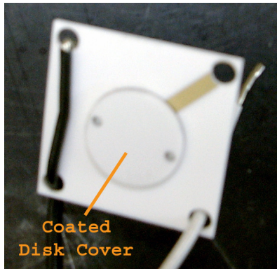
Figure 4: A different design trying to get good contact between the anode and cathode and their respective wires.
