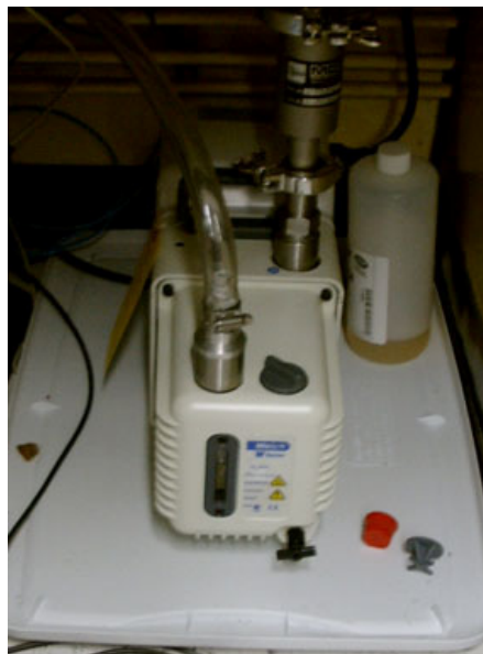
Figure 17: Direct drive rotary vane vacuum pump used in the backfilling system.
