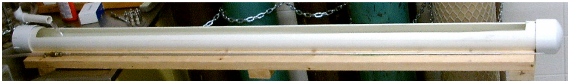
Figure 20: Long water tank used for leak checking each flux probe tube.
