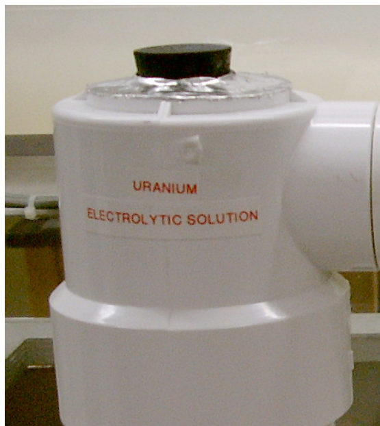
Figure 11: Sensor port for loading a pH and temperature sensor in the electrolytic flow path or for adding chemicals to the solution.
