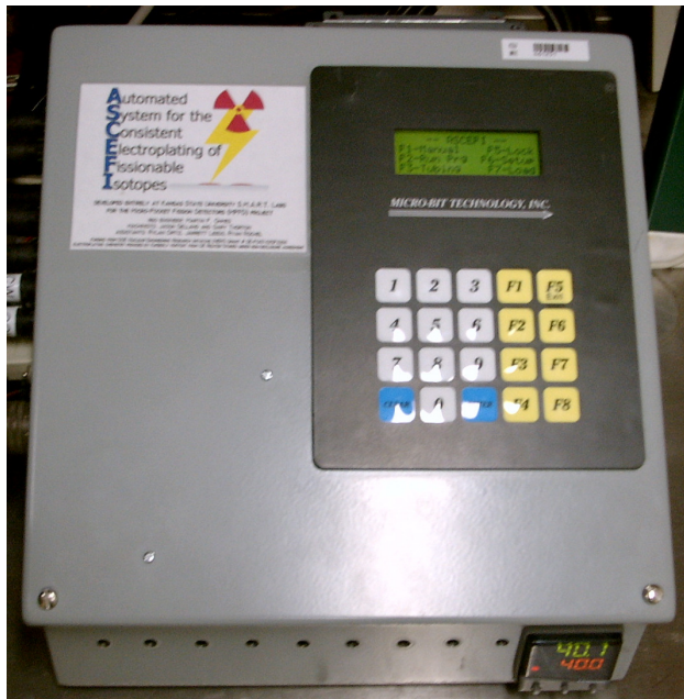
Figure 13: ASCEFI controller which monitors and controls all system components.
