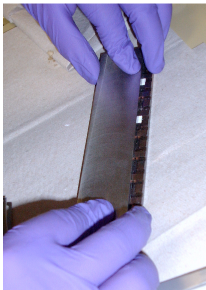
Figure 15: Interdigitated plates for aligning the substrate pieces and pressing them together.
