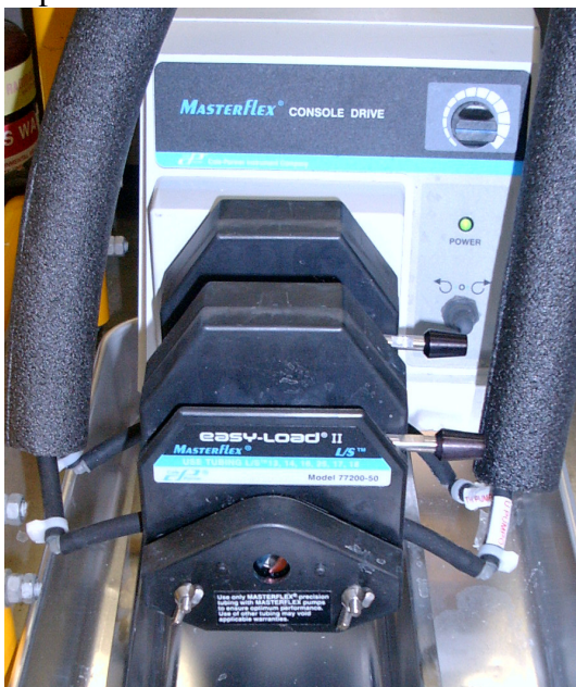
Figure 10: Peristaltic pump for controlling electrolytic solution flow.
