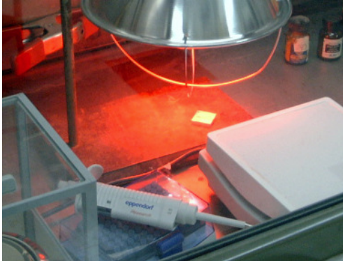
Figure 6: A uranyl nitrate drop is deposited on a substrate surface and dried under an infrared heat lamp.
