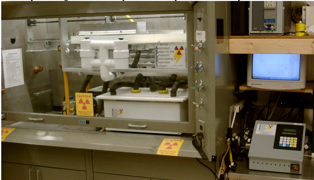
Figure 7: The Automated System for the Consistent Electroplating of Fissionable Isotopes.
