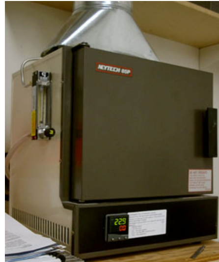
Figure 4: Nytech oven with new controller and inert gas injection line.
