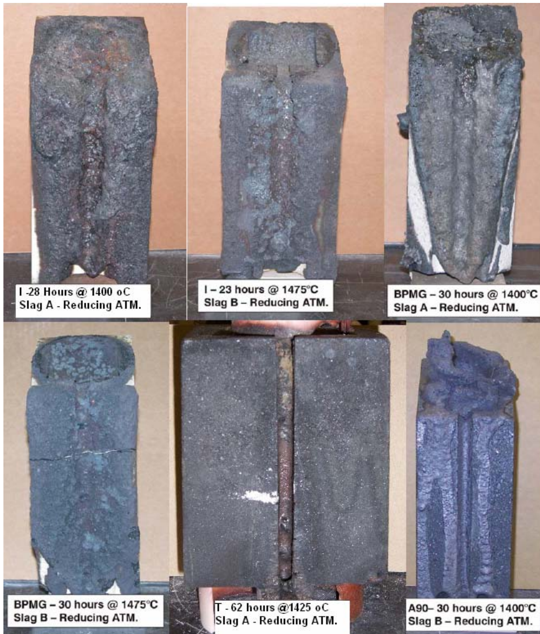
Figure 9. Bricks after the CADCAF Test.
