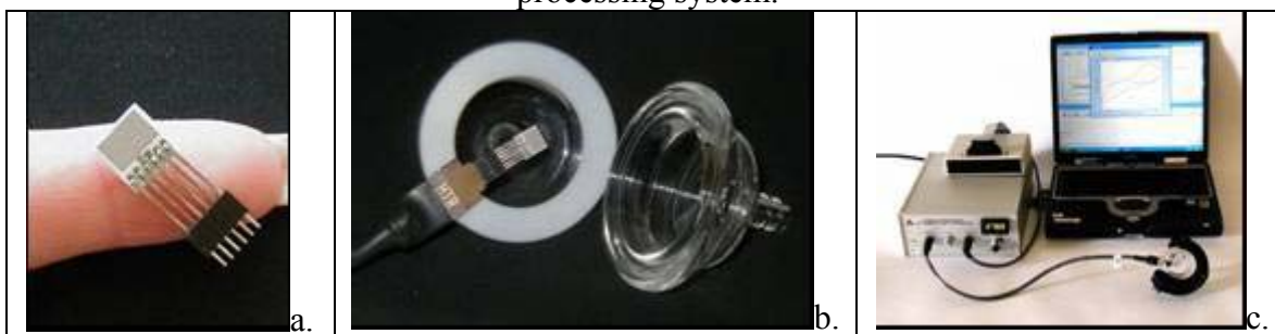
Figure 2. (a.) YSZ sensor, (b.) WBO sensor in enclosure, (c.) Complete testing and data processing system.
