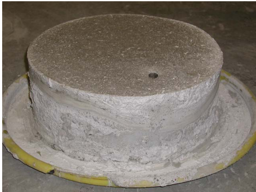
Figure 13 – CMS fiber concrete composite slab for nuclear shielding tests
