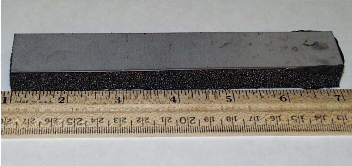
Figure 10. Foam-steel composite for flexural testing.
