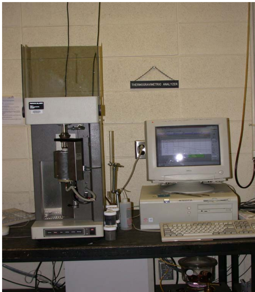
Figure 3. Picture of the PE-7A TGA apparatus used for the CO 2 studies.
