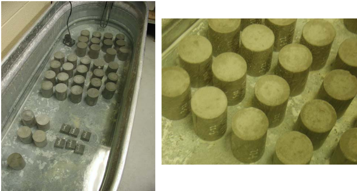
Figure 4 – Curing of concrete test specimens.
