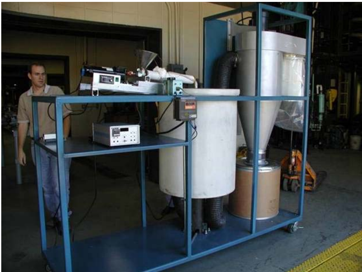
Figure 1 – Skid mounted CMS with cyclone collection system.
