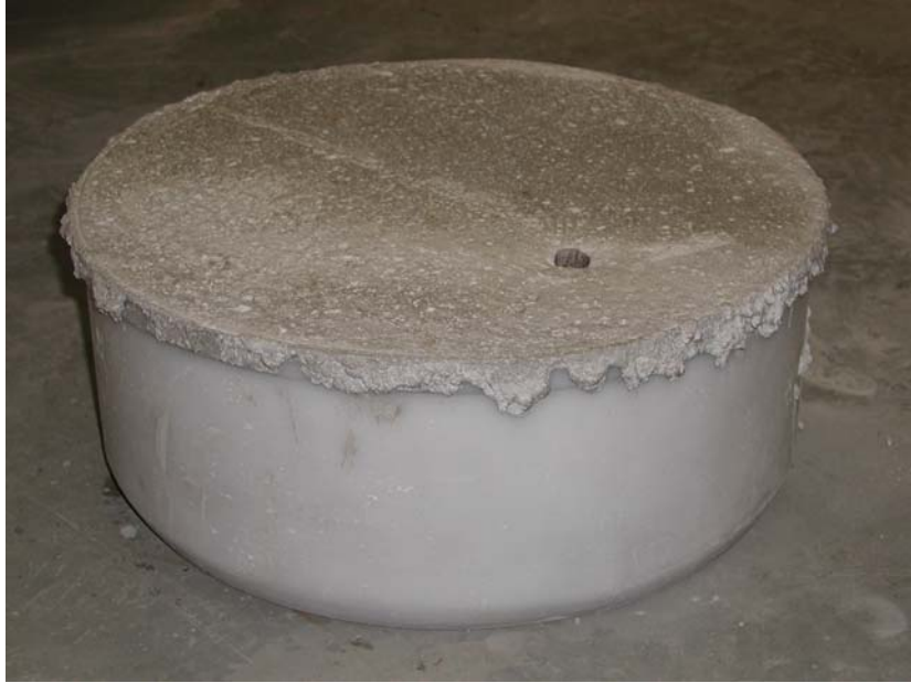
Figure 12 – Concrete slab for nuclear shielding tests
