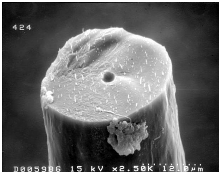
Figure 2 – W.Ky pitch fiber containing 2 wt% nanotubes.
