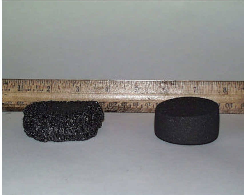
Figure 13. Carbon foam produced from SECO powder and CTP (right), and from CTP alone treated under the same conditions (left)
