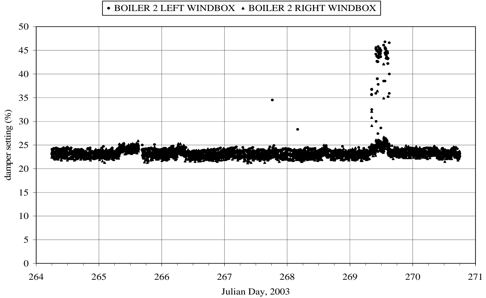
Figure D30. Air flow rates in left and right windbox, Boiler 2. Julian Day 264 = September 21, 2003.
