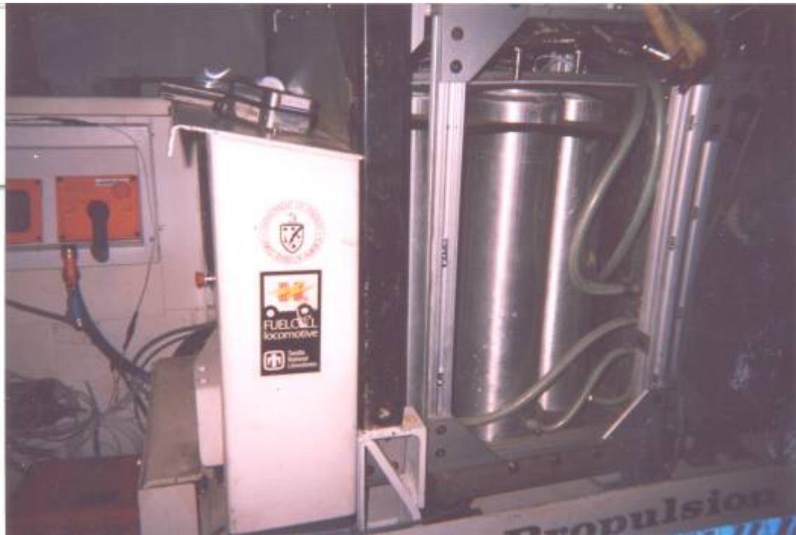
Exhibit 4. The hydride bed. Three of the 16 cylinders comprising the bed are visible.
