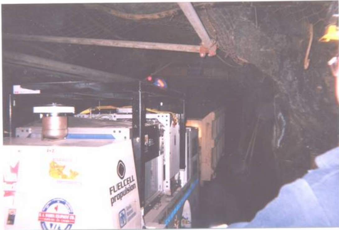
Exhibit 1. The fuel cell powered locomotive emerges from a tunnel, hauling three cars of gold ore.
