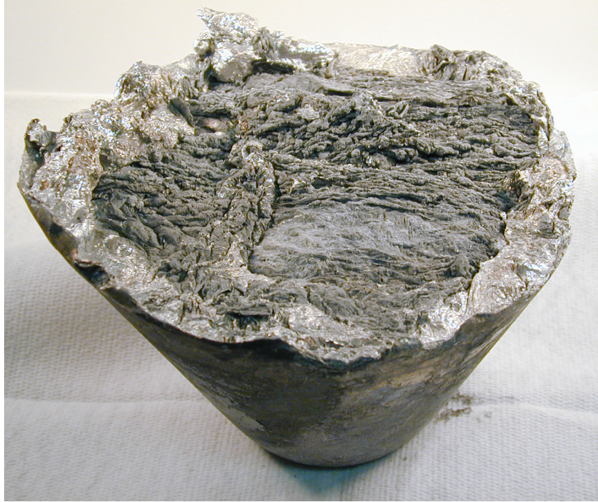
Fig 4.1: Bulk dross sample (~10-15 cm diameter at surface and 10 cm deep) after cooling and removing from crucible.
