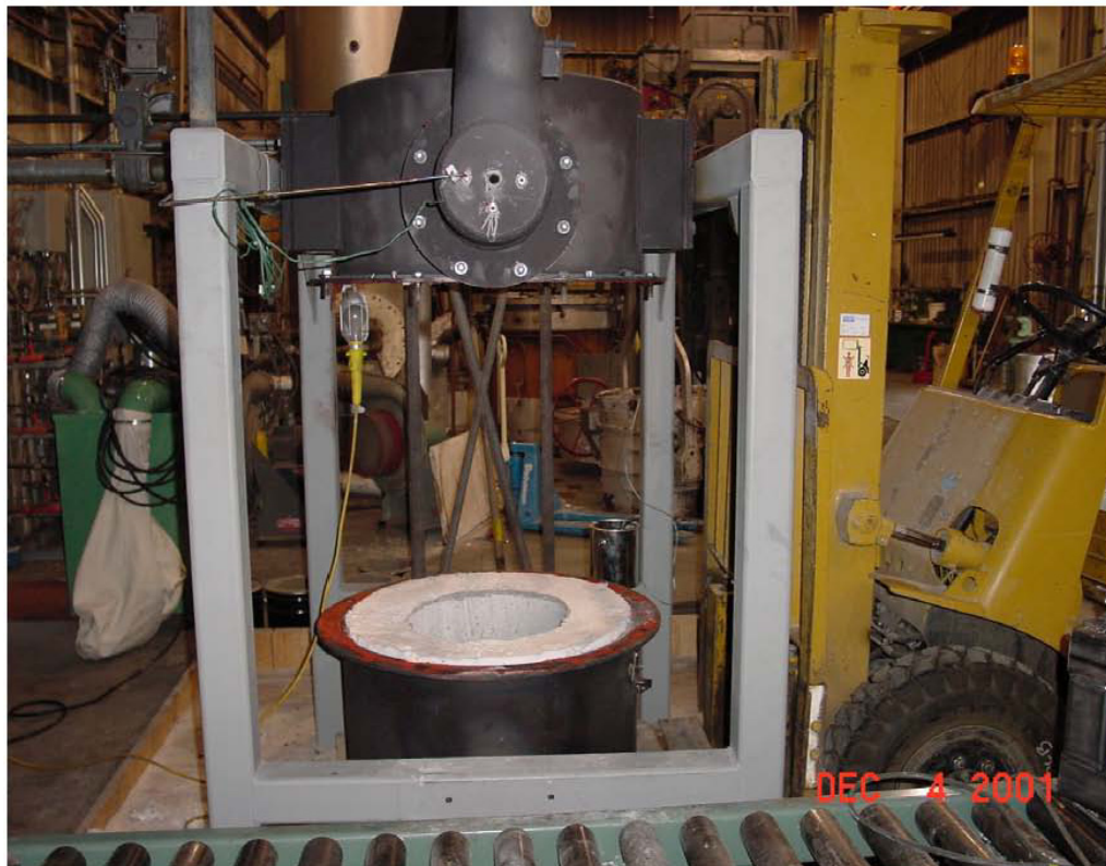
Fig 6.1: (Top) The ARC Laboratory Scale Reverb in operation during its inaugural heat. (Bottom) The ARC Laboratory Scale Reverb with the well and plenum sections separated in preparation for clean-up.
