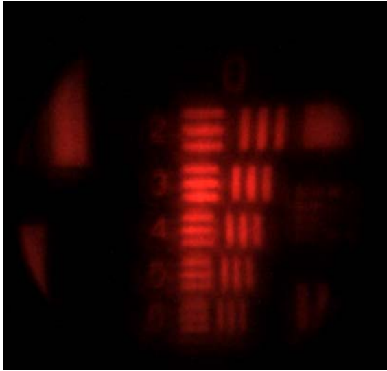
Figure 14. Images from transmissive nonmechanical zoom system using commercially available, liquid crystal lenses from OKO Technologies.
