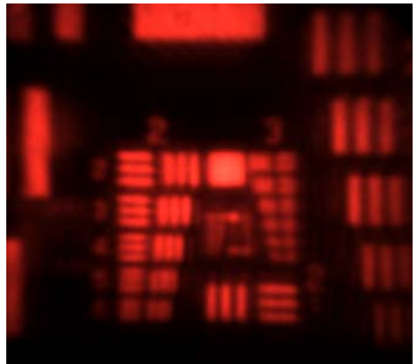
Figure 15. Images from transmissive nonmechanical zoom system using prototype liquid crystal lenses from HoloChip, Inc.
