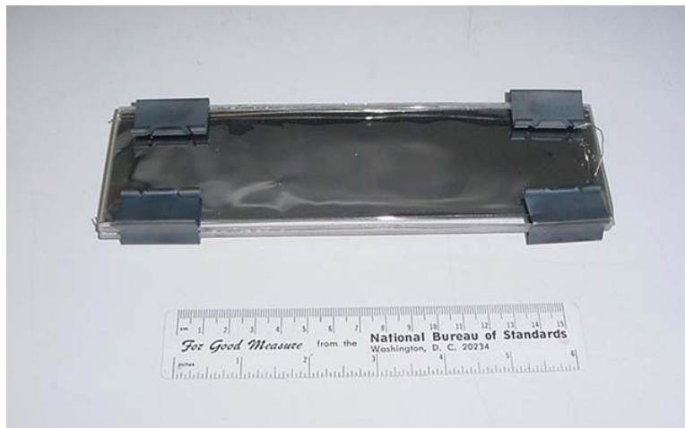
Figure 2. Photograph of fixture used to hold membranes flat during annealing.
