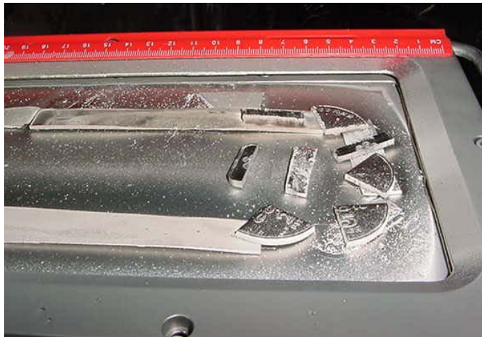
Figure 1. Sputter target modified to increase the membrane Pd content.
