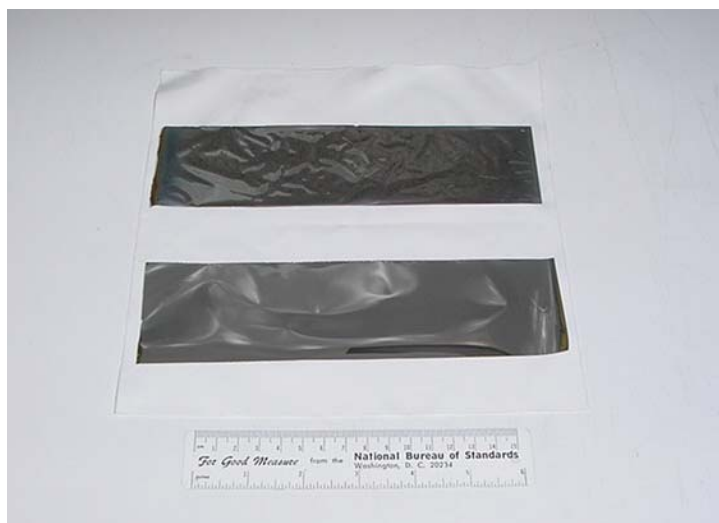
Figure 3. Full-size membranes before (foreground) and after (background) annealing in argon for 12 hours at 450°C.
