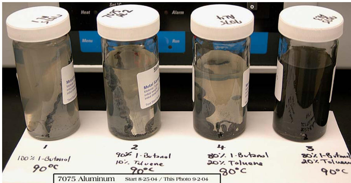
Figure 8. 7075 aluminum showing strong corrosion in the following four removal schemes: 80 °C 80 volume % 1-butanol / 20 volume % toluene, 90 °C 100% 1-butanol, 90 °C 90 volume % 1-butanol / 10 volume % toluene, and 90 °C 80 volume % 1-butanol / 20 volume % toluene. Corrosion began within 24 hours. No corrosion was observed with 40 °C furfuryl alcohol and 50 °C furfuryl alcohol after three weeks of exposure.
