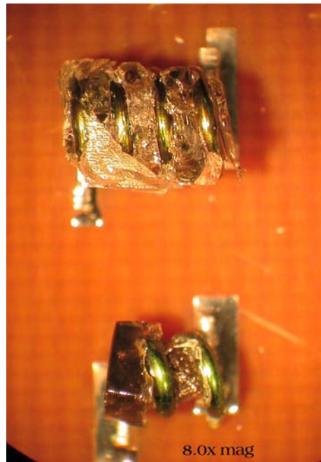
Figure 13. Encapsulated coil components shows partial dissolution of the components encapsulation after exposure to any of the four tested removal schemes.
