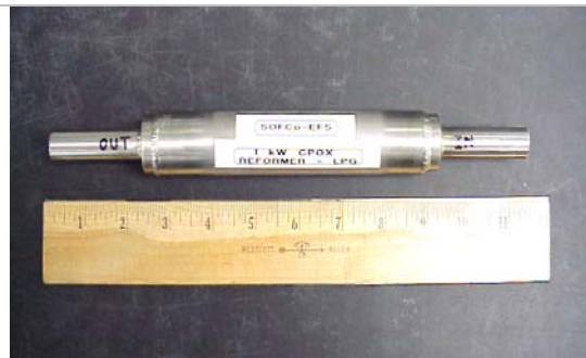
Figure 43. 1.5 kW CPOX reformer
