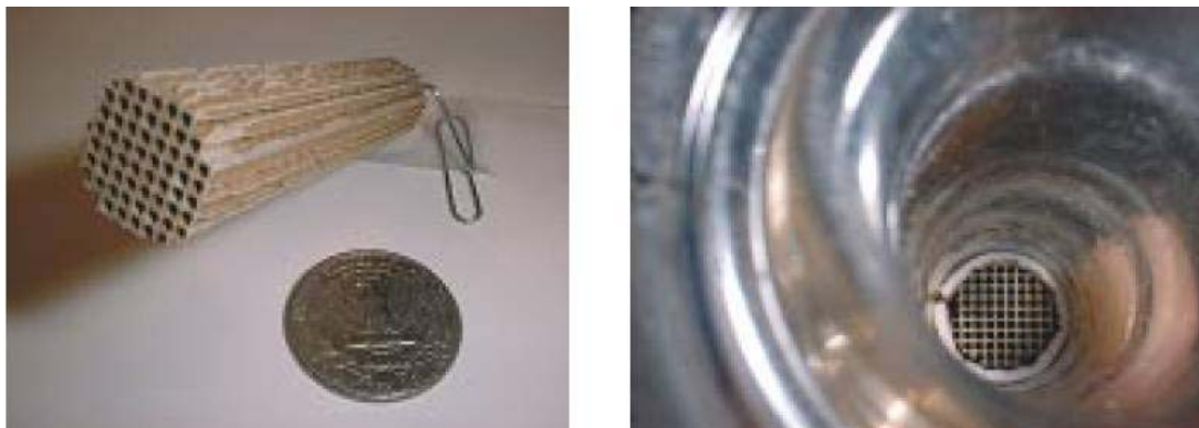
Figure 35. Monolith catalyst (left) and quartz reactor top view (right)
