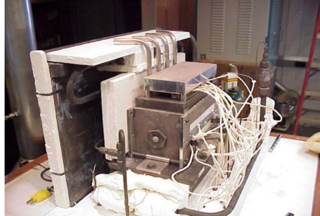
Figure 18. 47-cell stack in test stand
