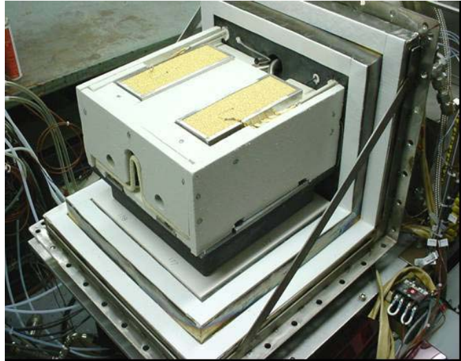
Figure 54. Stacks (2) installed and insulated in C1 hot box
