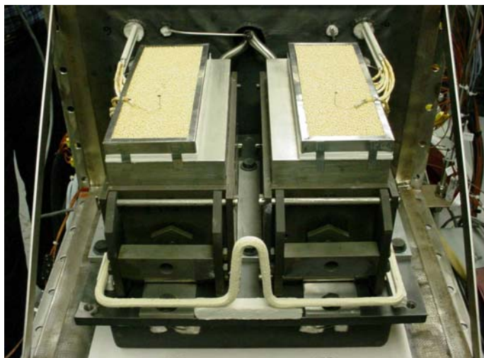
Figure 23. Two 48-cell stacks installed in the C1 module
