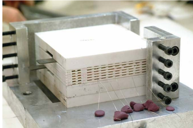
Figure 8. Typical 5-cell short stack
