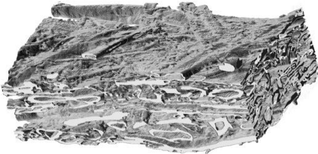
Figure 35: High-resolution 3D image of a newsprint sample.
