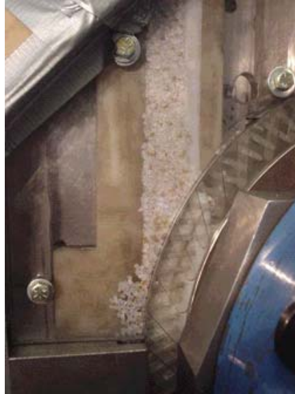
Fig.15 Flow Visualization Testing with Plastic pellets.
