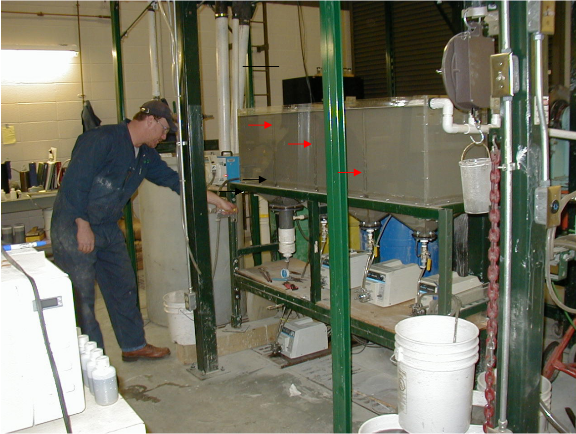
Figure 4. Photo of open channel hydraulic classifier with weirs.
