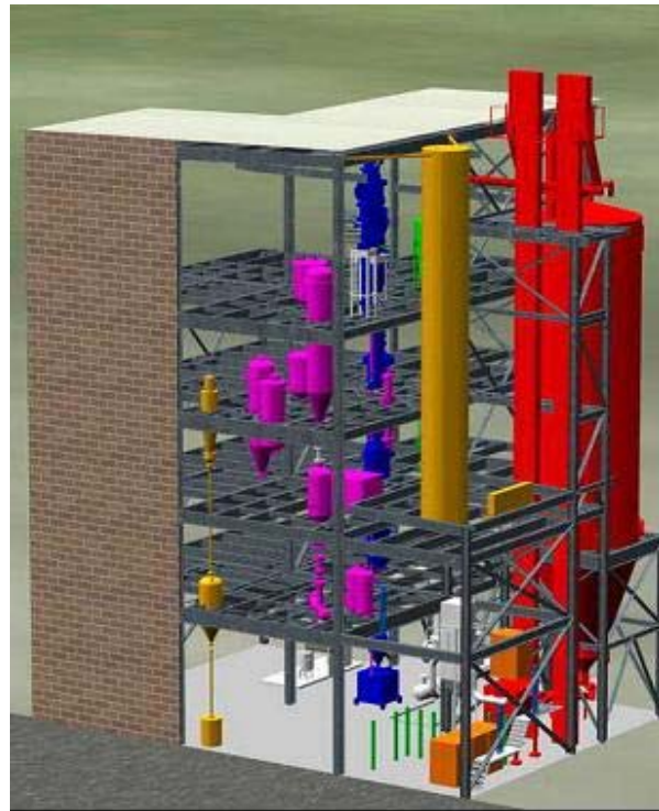
Figure 8 - Cutaway View of the FFTF Showing Solids Storage and Handling (Red), Gasification and Syngas (Blue), and NGC Process (Purple) Equipment
