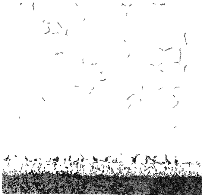
FIGURE 16. PRESSURE-BONDED SPECIMEN WITHOUT BARRIER LAYER
