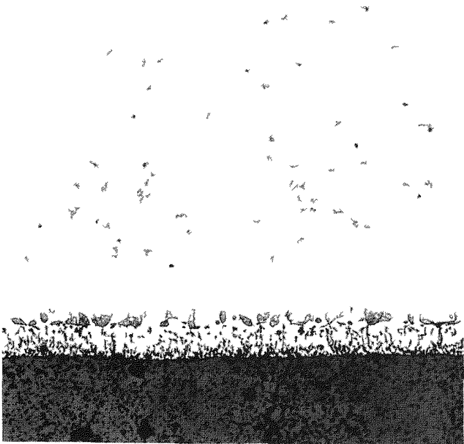
FIGURE 17. PRESSURE-BONDED AND HEAT-TREATED SPECIMEN WITHOUT BARRIER LAYER
