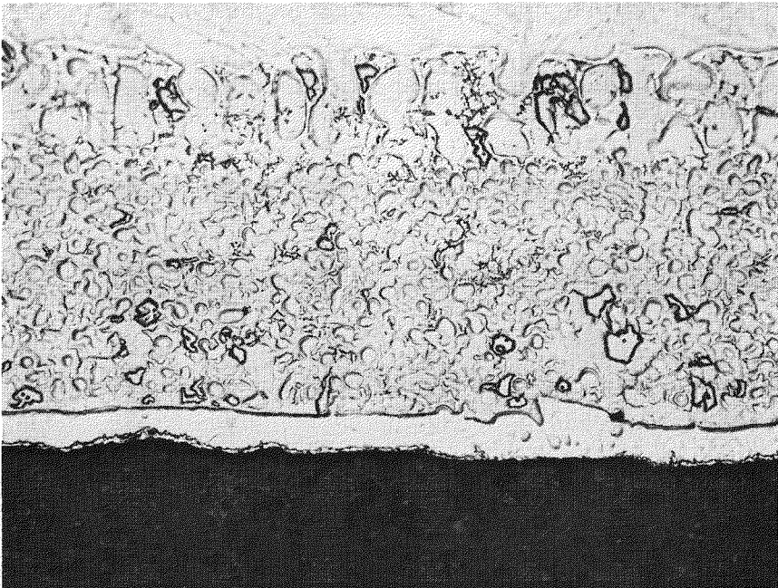
FIGURE 22. HEAT-TREATED SPECIMEN WITH IRON BARRIER LAYER
