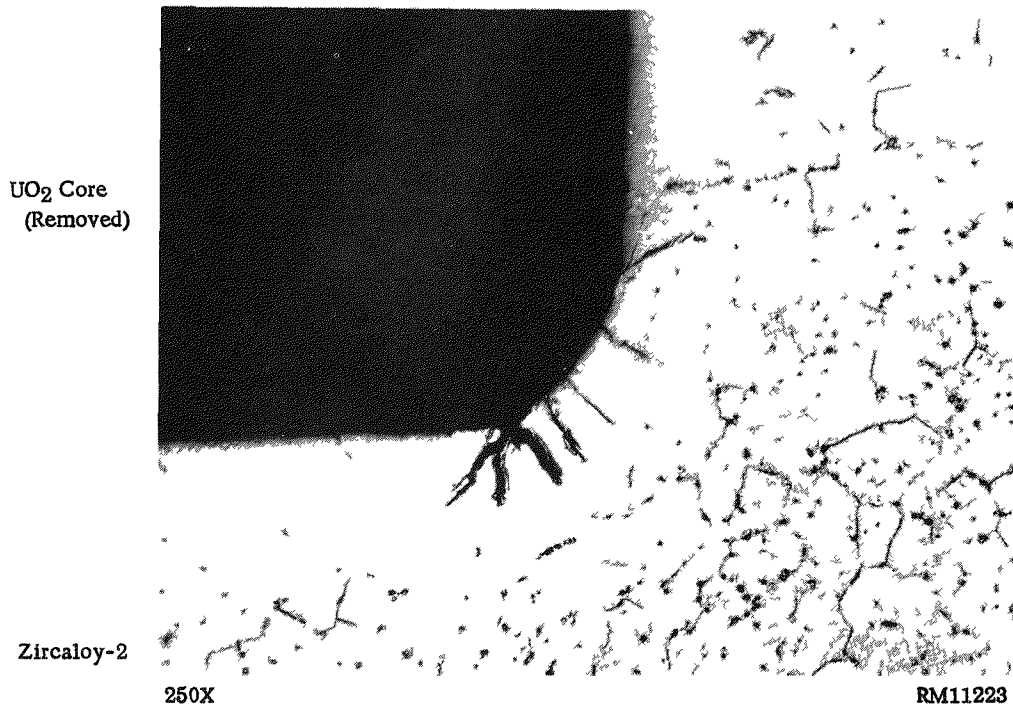
FIGURE 36. CRACKS AT A CORNER OF A GRAPHITE-COATED CORE
