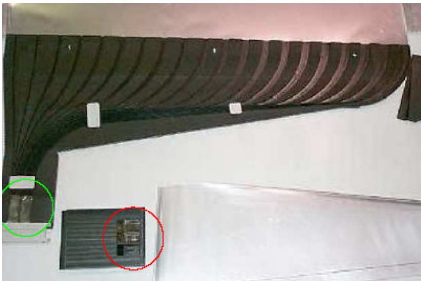
Figure 6.7: Prototypes of the ashtray and readout fibre pigtails in a FarDet module. The LI fibre connects into the ashtray (circled in red) and illuminates the readout fibres on the module (green) [65].
