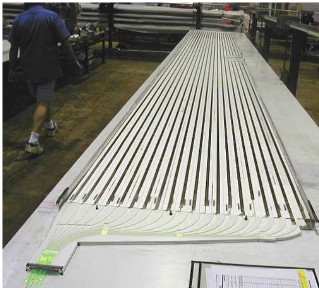
Figure 3.6: The inside of a FarDet scintillator module during construction. The strips can be seen running along the length of the module. The scintillator modules are then encased in 0.5 mm thick aluminium and attached to the steel planes.
