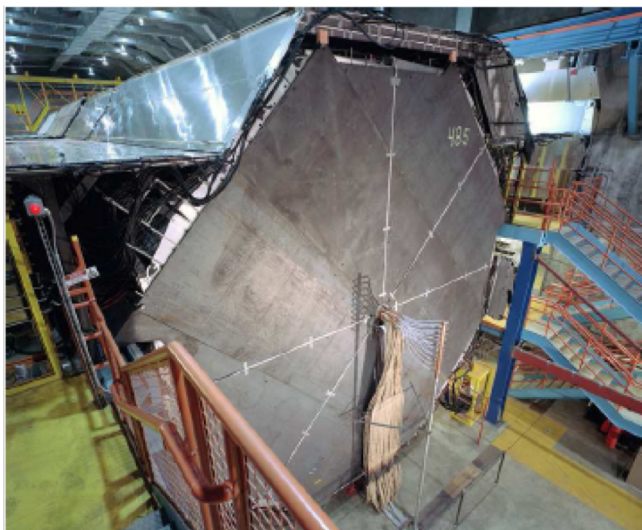
Figure 3.14: The face of FarDet, showing the last steel plane where the neutrino beam exits. The veto shield can be seen covering the top of the detector. [Photo: Jerry Meier.]
