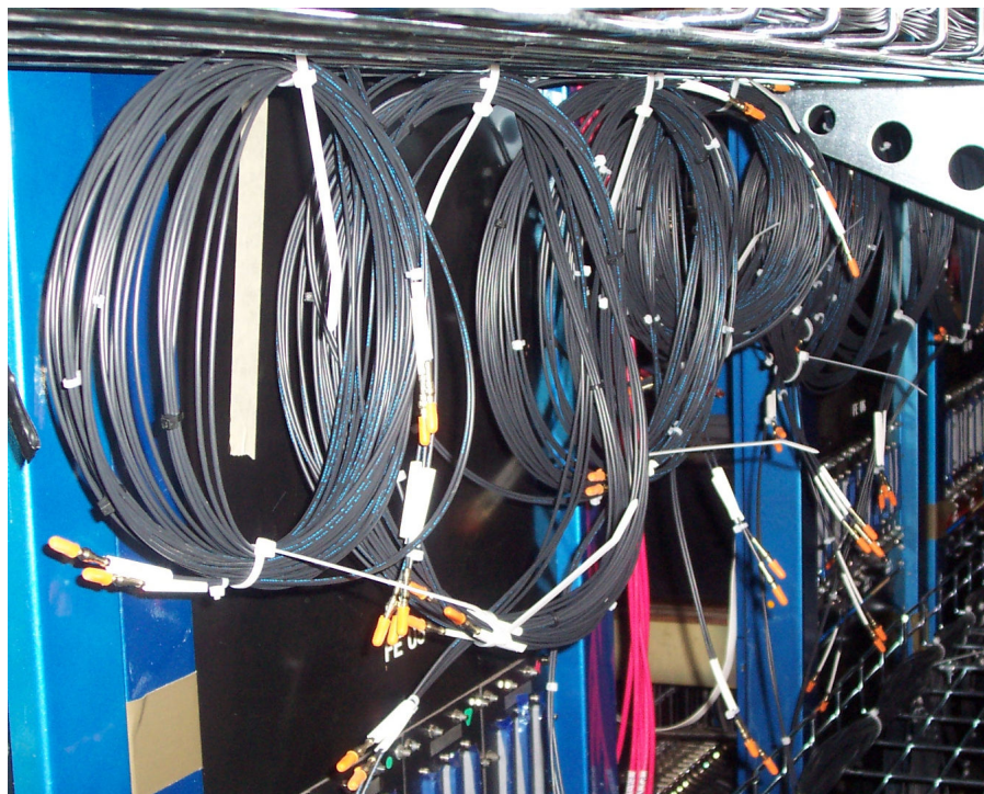
Figure 6.6: Sets of LI fibres at NearDet, where the fibres were connected to the pulser boxes before installation to the planes (this was done the other way around during FarDet installation). Orange rubber protects the optical output end of the fibres, which shines on the readout fibres.
