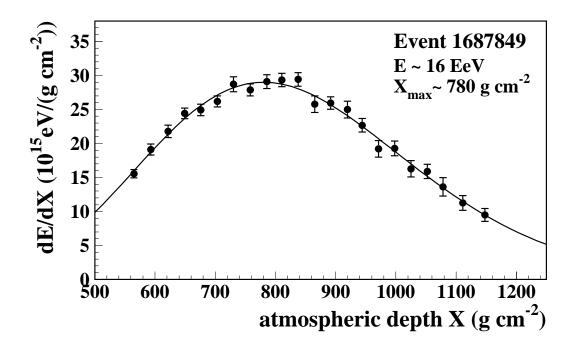
Fig. 4. Example of a reconstructed longitudinal energy deposit profile (points) and the fit by a Gaisser-Hillas function (line).
