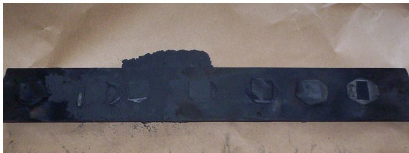
Figure 45: Free carbon deposited on samples after carburization
