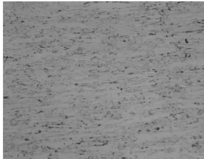
Figure 12. Showing Optical Micrograph of Extruded (10:1) Iron Aluminide Longitudinal (200X)
