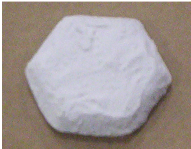
Figure 44: Side view show Thermal Sprayed Sample one face is exposed, other faces are covered in Alumina
