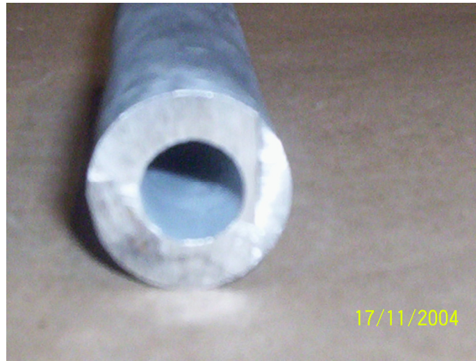
Figure 7: Showing alumina reinforced iron aluminide tube fabricated by CIP/sinter process and net shape component by powdermetallurgy technique demonstrated using this CVD coated powder
