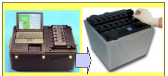
The LLNL Advanced Nucleic Acid Analyzer demonstrated 7 minute PCR detection in April 1999. LLNL technology licensed to Cepheid helped create the Smartcycler product that is now used in LLNL field labs.
