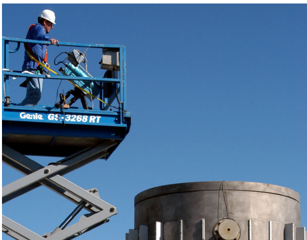
Fig. 2. Gamma-ray imager looking down on the MC-10 cask.
