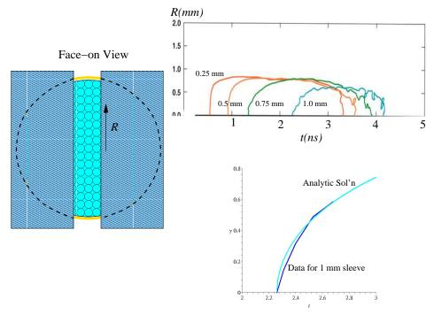
Data from the 0.8 mm radius and 1 mm long Au sleeve (optically thick case) experiment is well matched with  $D = 0.46 \text{ mm}^2/\text{ns}$  and  $\varepsilon = 0.3$ –providing a measure of wall albedo.
