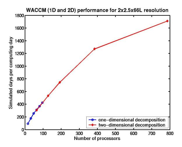
Fig. 9. Throughput (in simulated days per computing day) of the 2° x 2.5° x 66L resolution with 51 constituents on the IBM SP with Nighthawk 16-way nodes, as a function of processor count. This configuration is typical of the Whole Atmosphere Community Climate Model (WACCM). The two-dimensional domain decomposition increases the throughput four-fold as compared to the one-dimensional decomposition.
