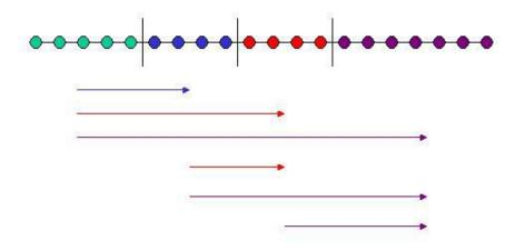
Fig. 4. Partial sum methodology for geopk. The atmospheric levels (here illustrated in the horizontal) are distributed over DE's. When integrating vertically upward, each DE does a local integration in parallel and passes its result to all DE's above it. Bitwise reproducibility, if desired, can be ensured through use of high precision arithmetic.
