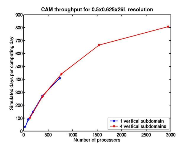
Fig. 8. Throughput (in simulated days per computing day) of the  $0.5^{\circ}$  x  $0.625^{\circ}$  x 26L resolution on the IBM SP with Nighthawk 16-way nodes, as a function of processor count. The leftmost curve is with 1 subdomain in the Z direction (up to 736 processors), and the longest curve is with 4 subdomains in the Z direction (up to 2944 processors). All cases use 8 OpenMP threads per process.
