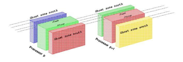
Fig. 1. The one-dimensional algorithm decomposes the latitude-longitude-level domain into a set of latitudinal slabs. Each slab, or decomposition element (DE), has a north and south halo region, which covers the latitudinal data dependencies. These halo regions are filled  $(halo\ exchange)$  before  $cd\_core$  calculations in a communication phase that can be overlapped with unrelated computation. The calculation on haloed arrays can then take place without further communication.
