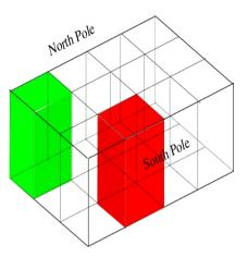
Fig. 2. The two-dimensional domain decomposition formulation requires different decompositions for different phases of the computation. A decomposition in latitude and level (left) is used for dynamics and transport within a control volume, whereas a decomposition in longitude and latitude (right) is used for the surface remapping. The two decompositions are connected by optimized transposes.
