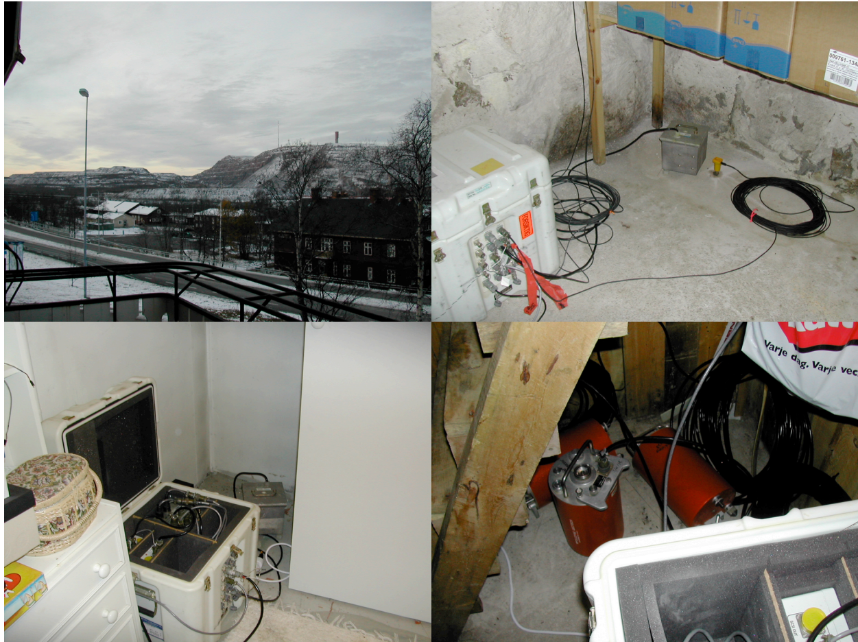
Figure 6. Photographs of Kiruna and Malmberget deployments. The historic surface mine is apparent as the gap in the hill in the photograph at top left. Today the ore is mined underground. The collocated S6000 and geophone in array 2 at Kiruna are shown in the upper right photograph. A typical Malmberget deployment in the basement of a private home is shown at lower left. Station ALN is shown at lower right.
