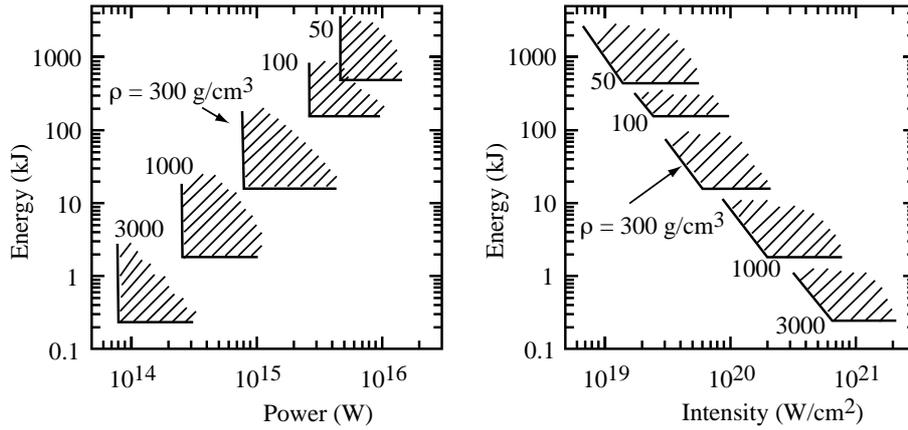
**Figure 1.** Fast ignition windows, for different values of the fuel density.
