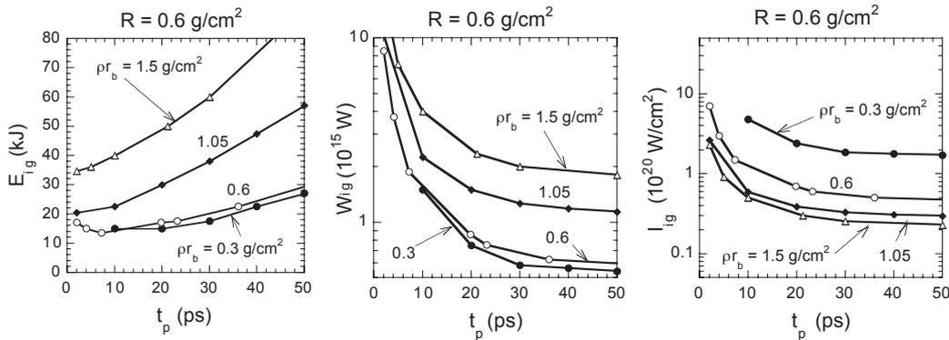
**Figure 2.** Ignition energy, power, intensity, vs pulse time, for different values of the beam radius, and the same penetration depth  $\mathcal{R} = 0.6 \text{ g/cm}^2$ .
