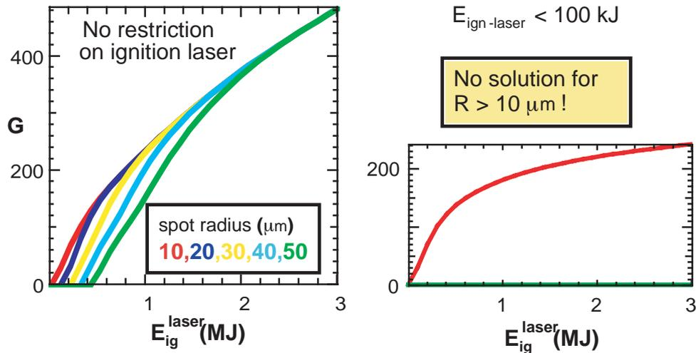
**Figure 5.** Gain vs total laser energy for different values of the ignition laser spot size, for the parameters given in the main text. a) with no constraints to the ignition laser energy; b) with ignition laser energy limited to 100 kJ.
