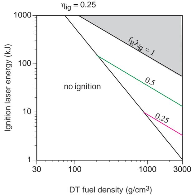
**Figure 3.** Laser ignition energy for hot-electron driven fast ignition vs density of the precompressed fuel, for different values of the parameter  $f_{\mathcal{R}} \hat{\lambda}_{\text{ig}}$ .
