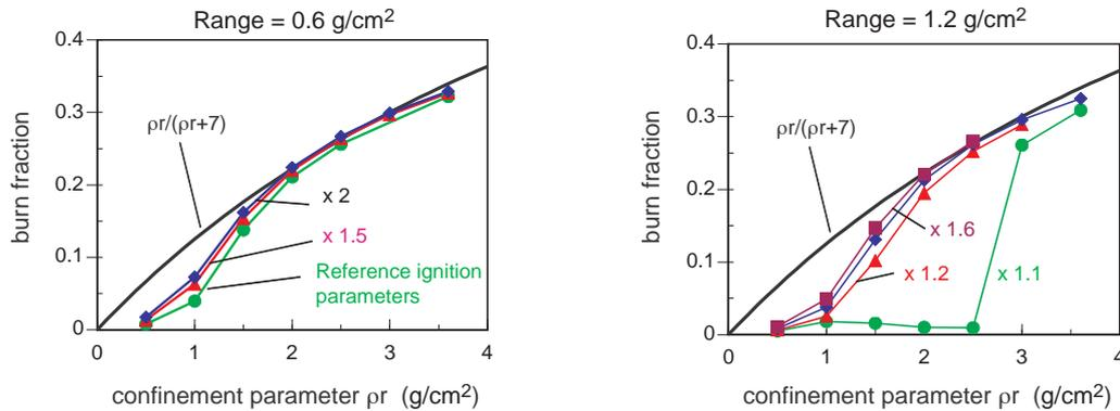
**Figure 4.** Burn efficiency vs confinement parameter, for different ranges and different ignition pulse parameters.
