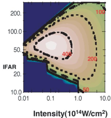
**Figure 6.** Gain contours in the IFAR-compression laser intensity plane, for total laser energy of 3MJ; focal spot limited to 10  $\mu\text{m}$ ;  $f_{\mathcal{R}}\hat{\lambda}_{\text{ig}} = 1$ .
