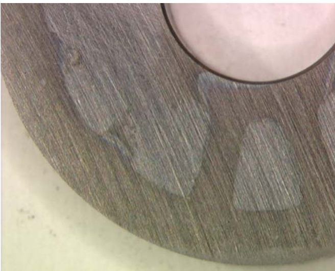
FIGURE 18 – Specimen JE3380, MA polished Alloy 22 after CPP in 0.1 m NaCl + 0.001 m NaHCO 3 at 60°C
