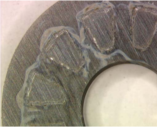
FIGURE 16 – Specimen JE3381, MA polished Alloy 22 after CPP in 0.1 m NaCl + 0.001 m NaHCO 3 at 95°C
