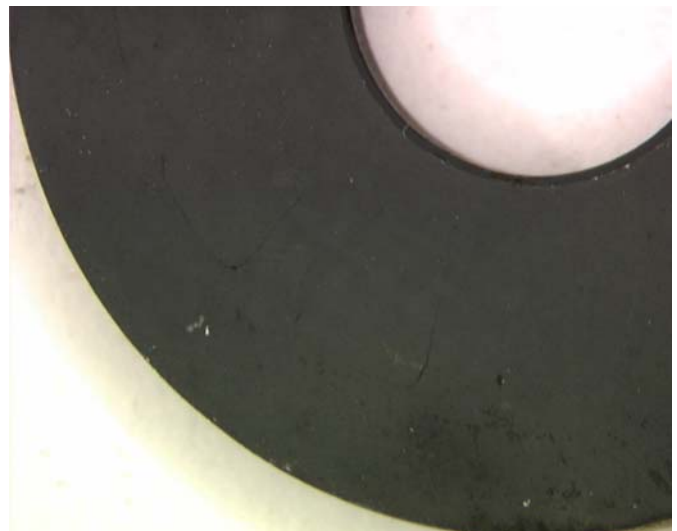
FIGURE 19 – Specimen JE3372, SHT Alloy 22 after CPP in 0.1 m NaCl + 0.001 m NaHCO 3 at 60°C
