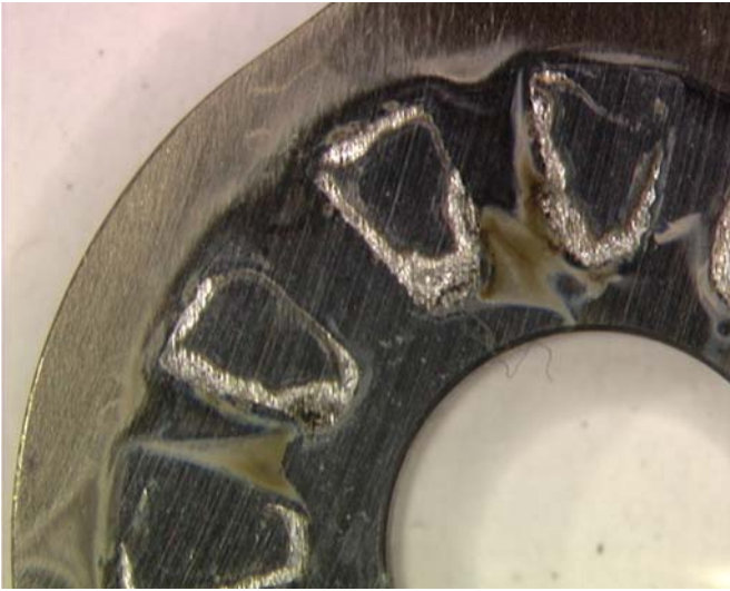
FIGURE 12 – Specimen JE3315, MA Alloy 22 after CPP in 6 m NaCl + 0.3 m KNO 3 at 100°C
