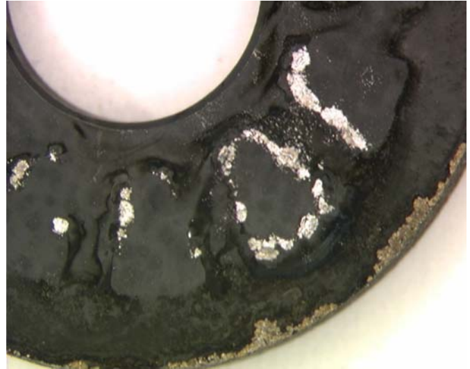
FIGURE 17 – Specimen JE3373, SHT Alloy 22 after CPP in 0.1 m NaCl + 0.001 m NaHCO 3 at 95°C
