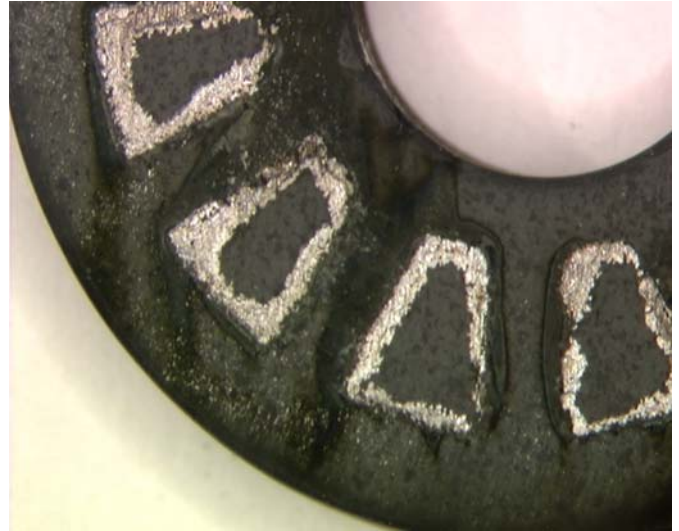
FIGURE 13 – Specimen JE3308, SHT Alloy 22 after CPP in 6 m NaCl + 0.3 m KNO 3 at 100°C
