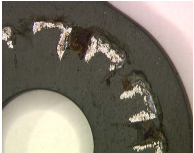
FIGURE 11 – Specimen JE3303, SHT Alloy 22 after CPP in 1 M NaCl at 90°C
