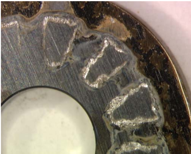
FIGURE 10 – Specimen JE3328, MA polished Alloy 22 after CPP in 1 M NaCl at 90°C
