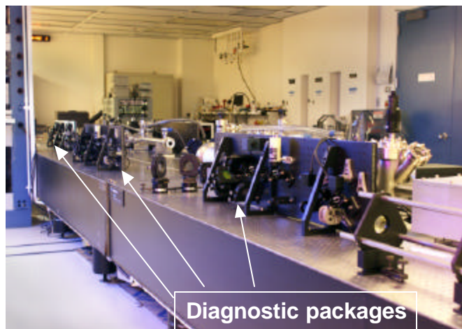
Fig. 2.1.4.1 A view showing the small footprint of the vertically mounted diagnostic packages next to the Mercury laser beamline
