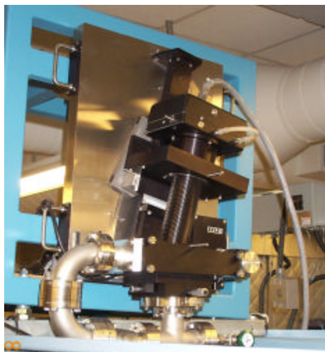
Fig. 2.3.3.2 X-rays are collected with an ellipsoidal condensing optic and directed vertically upwards towards the target. When the target is rotated out of view, the soft x-ray spectrometer has a direct view of the plasma.
