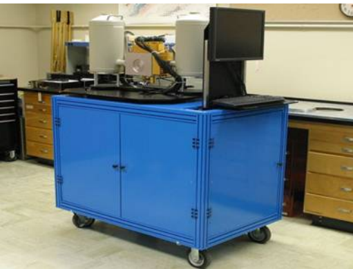
Fig. 3: The integrated mobile hybrid Compton imaging platform.
