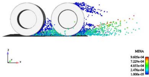
Figure 2: Droplet dispersion about tandem dual tire
