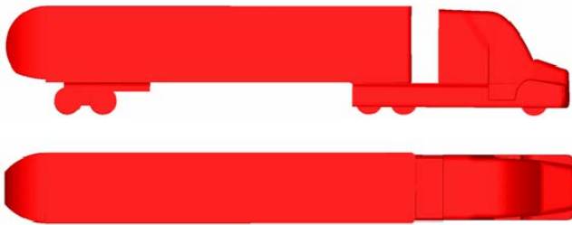
Figure 18. Modified GCM Geometry with Aerolution's Inflatable Boat Tail Device.
