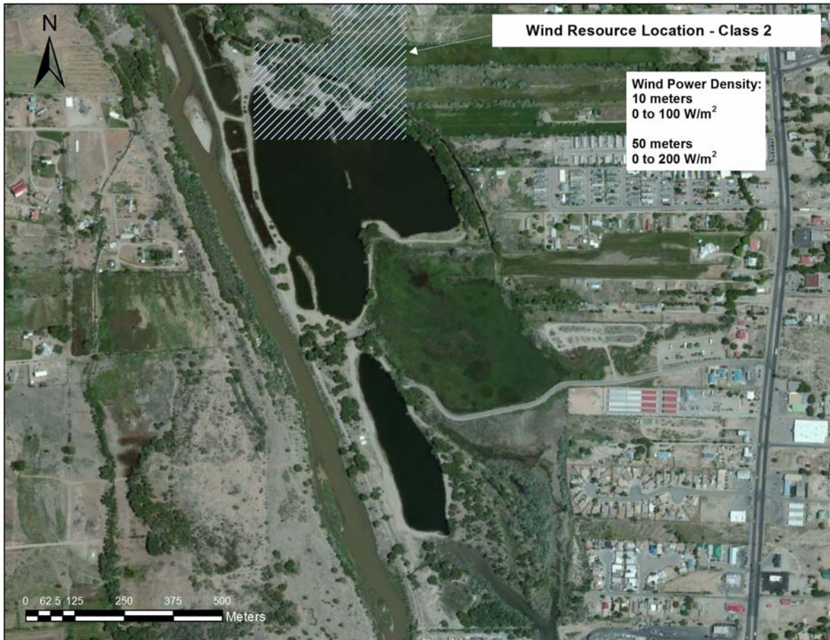
Figure 10. Wind resource potential from the National Renewable Energy Laboratory database at the ByWater Lakes site.
