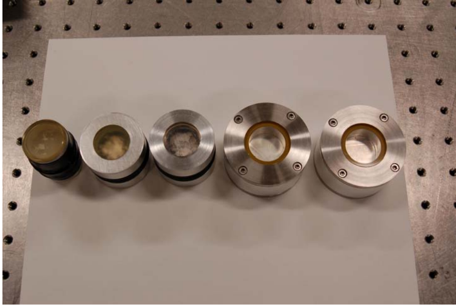
Figure 2.1. Five tested detectors using Li foil interfaced with an alkali halide scintillator. Good hermetic sealing was needed to achieve stable detectors with no degradation of the Li foil.
