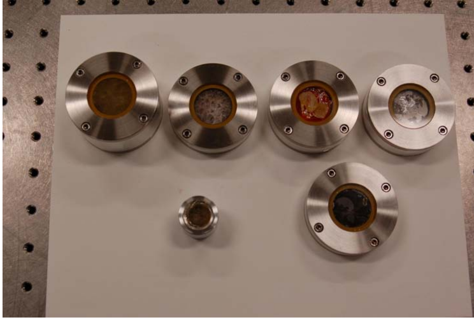
Figure 2.2. Polycrystalline NaI(Li,Tl) samples tested for thermal neutron sensitivity. Diverse color and transparency can be seen in these samples, indicating the sensitivity of the material to variations in the production process and dopant concentration.
