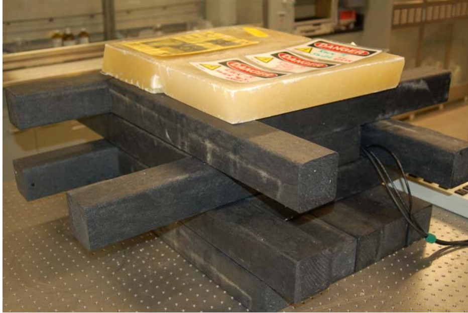
Figure 2.3. A cave was constructed of HDPE and paraffin to moderate the fission spectrum neutrons emitted from ^{252}\text{Cf} and increase the flux of thermal neutrons through the detector.
