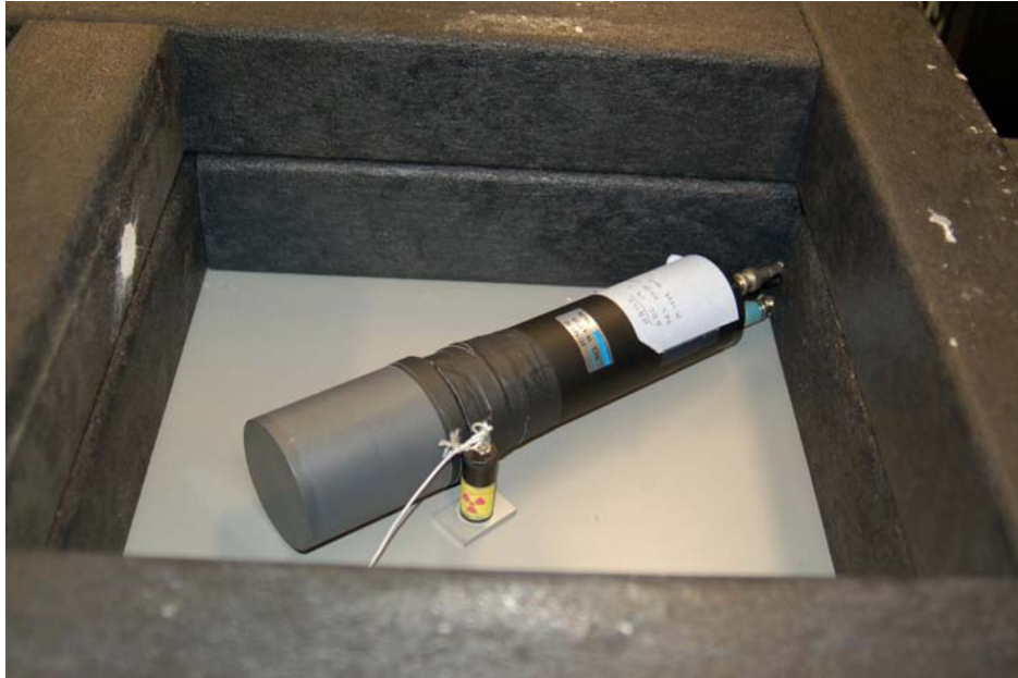
Figure 2.4. The ^{252}\text{Cf} source (cylinder with string attached) and the detector under test were placed in the center of the cave on an aluminum plate.
