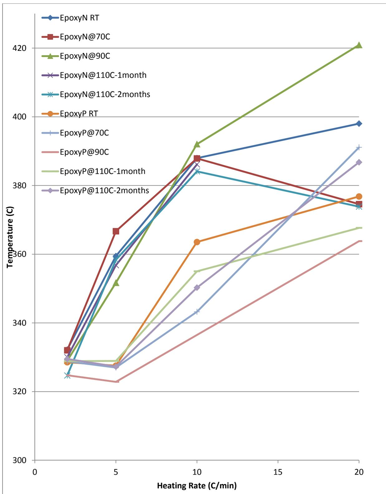
Figure 6: Temperature of peak calculated from the first derivative of heat flow using DSC. Mean of three experiments shown unless otherwise noted
