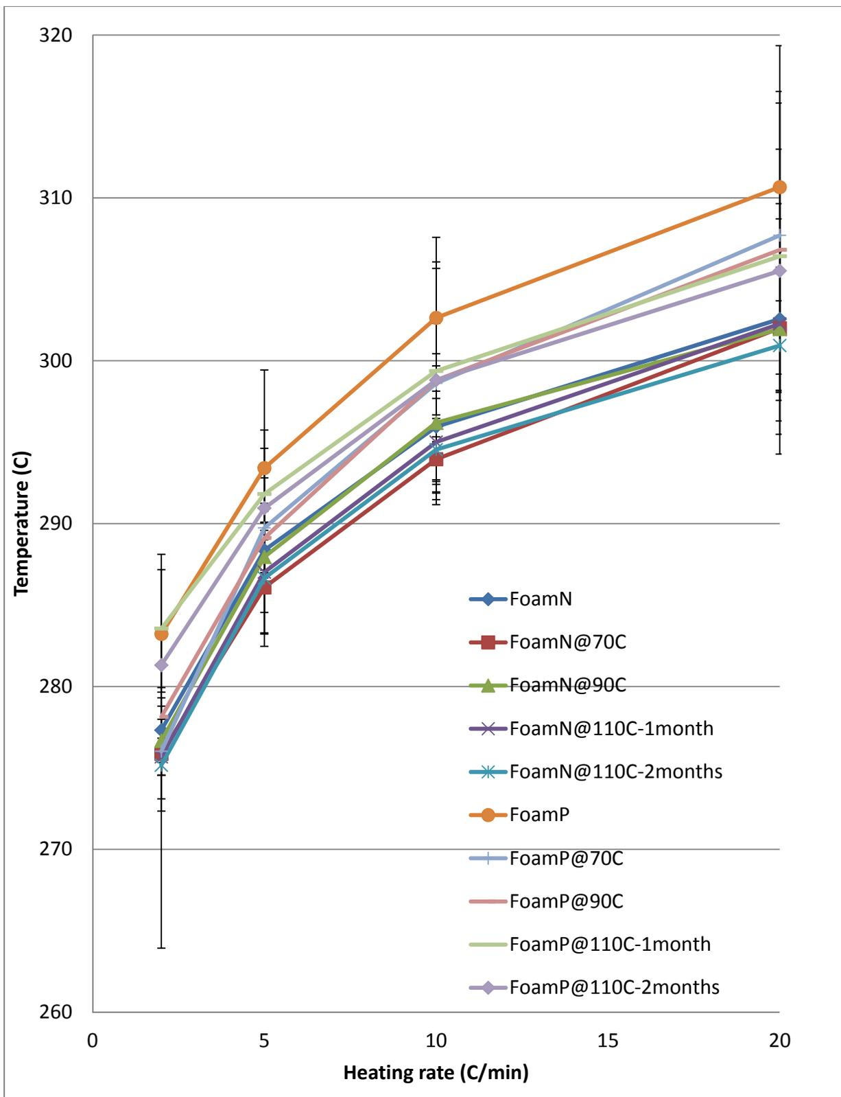
Figure 1: Averaged TGA data for foam materials at 10% weight loss. Means and 95% confidence intervals are plotted for three independent TGA measurements.
