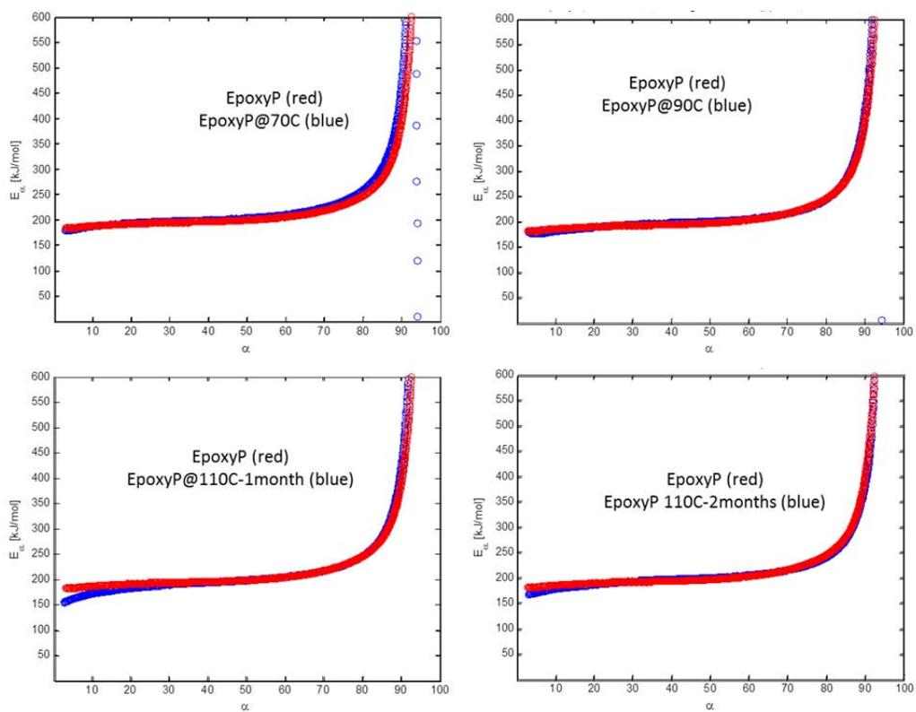
Figure 10: Apparent activation energy versus conversion ( $\alpha$ ) for EpoxyP.
