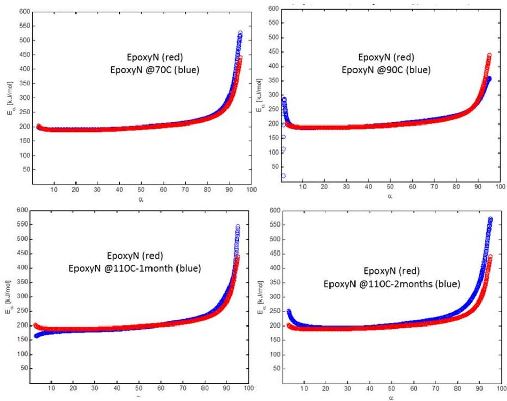
Figure 9: Apparent activation energy versus conversion ( $\alpha$ ) for EpoxyN.
