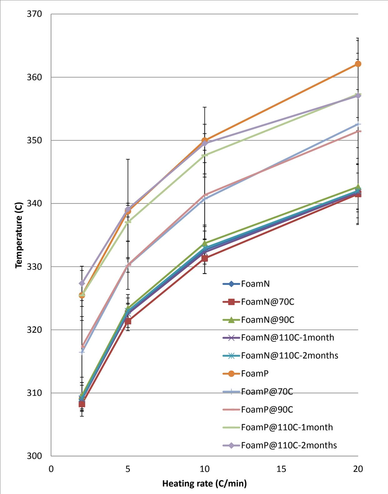
Figure 2: Averaged TGA data for foam materials at 50% weight loss. Means and 95% confidence intervals are plotted for three independent TGA measurements.
