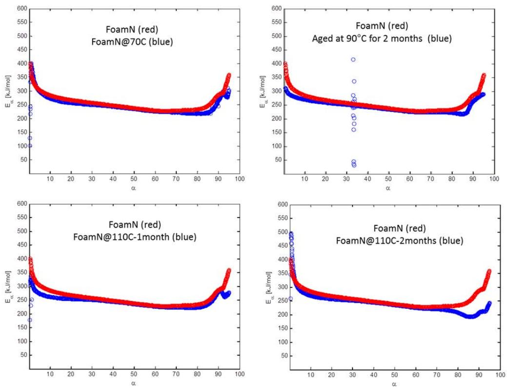
Figure 7: Apparent activation energy as a function of conversion ( $\alpha$ ) for FoamN.
