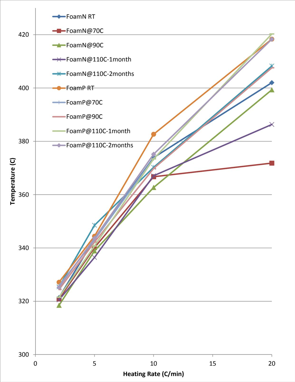
Figure 5: Temperature of peak calculated from the first derivative of heat flow using DSC. Mean of three experiments shown unless otherwise noted.
