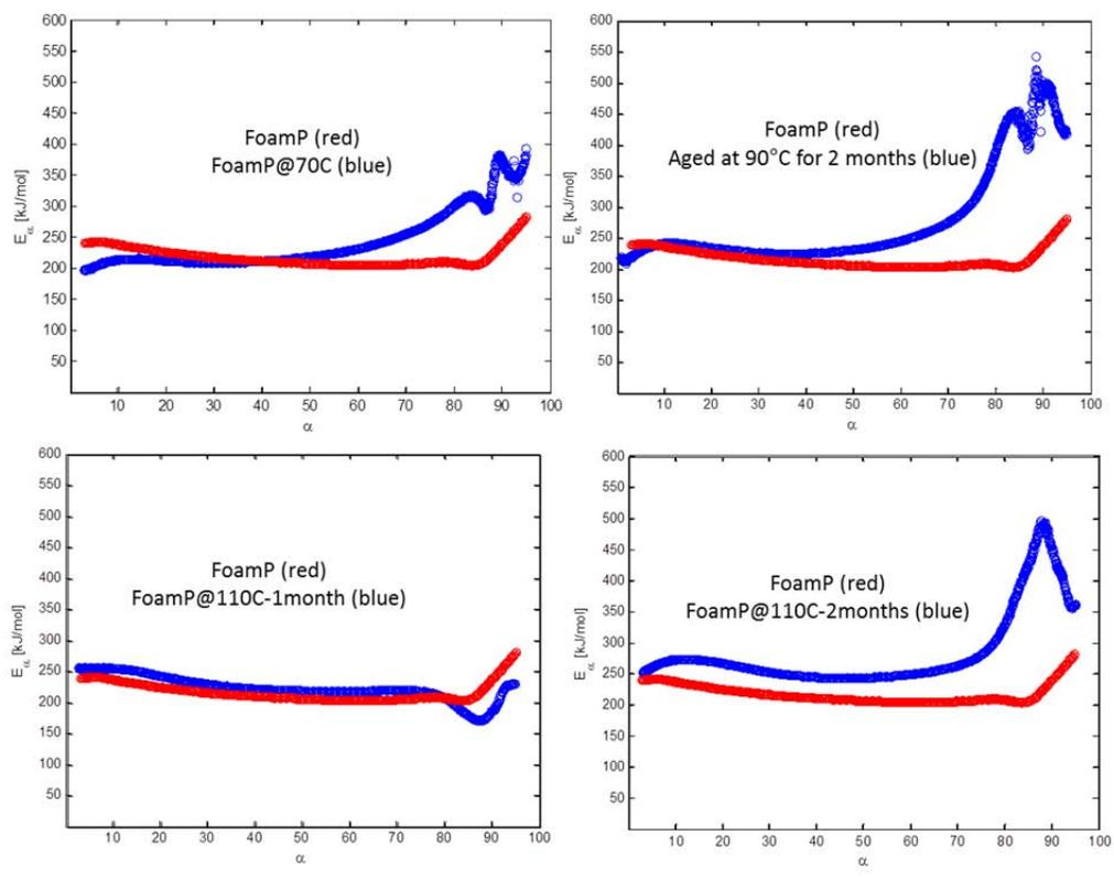
Figure 8: Apparent activation Energy versus conversion ( $\alpha$ ) for FoamP.
