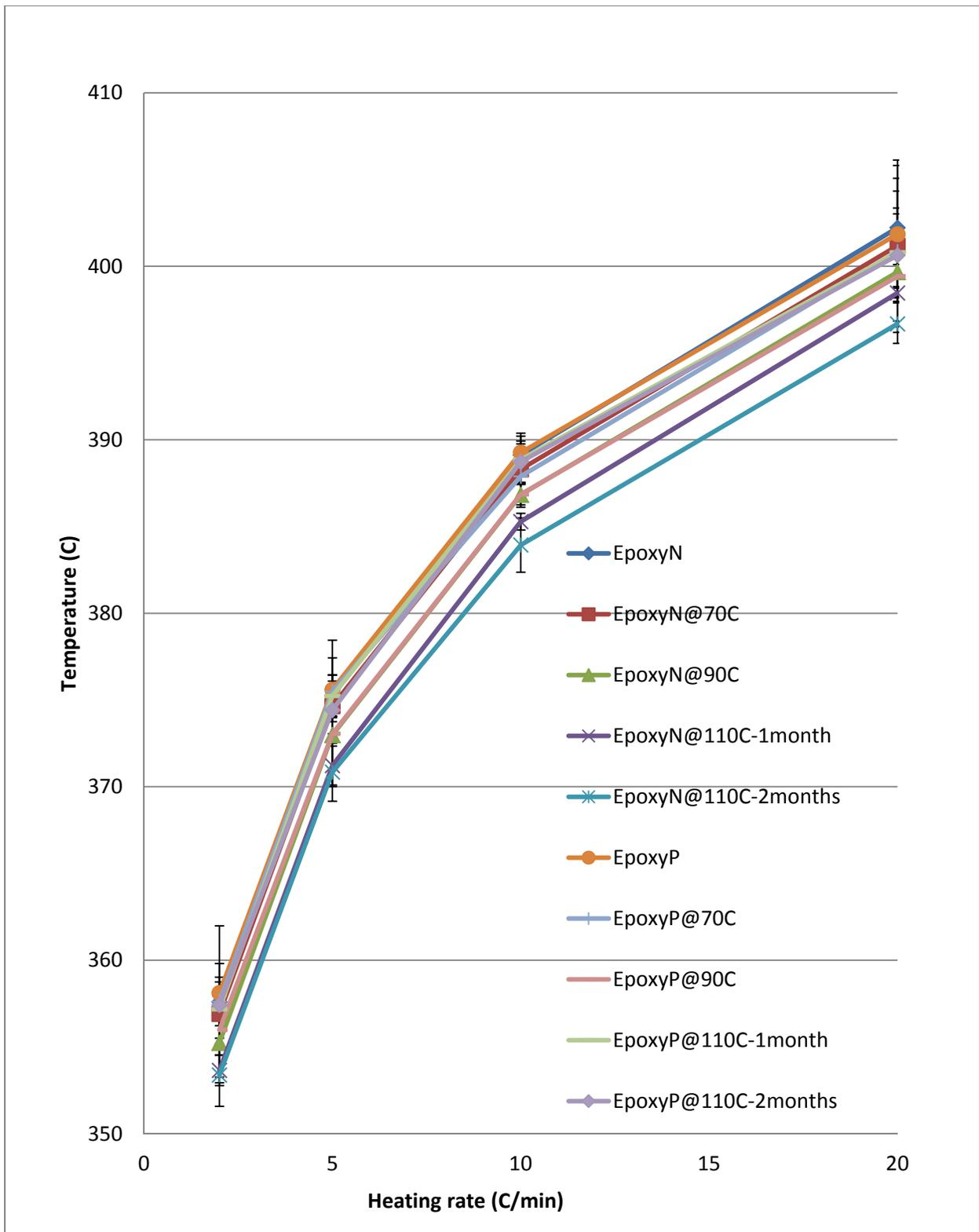
Figure 4: Averaged TGA data for epoxy materials at 50% weight loss. Means and 95% confidence intervals are plotted for three independent TGA measurements.
