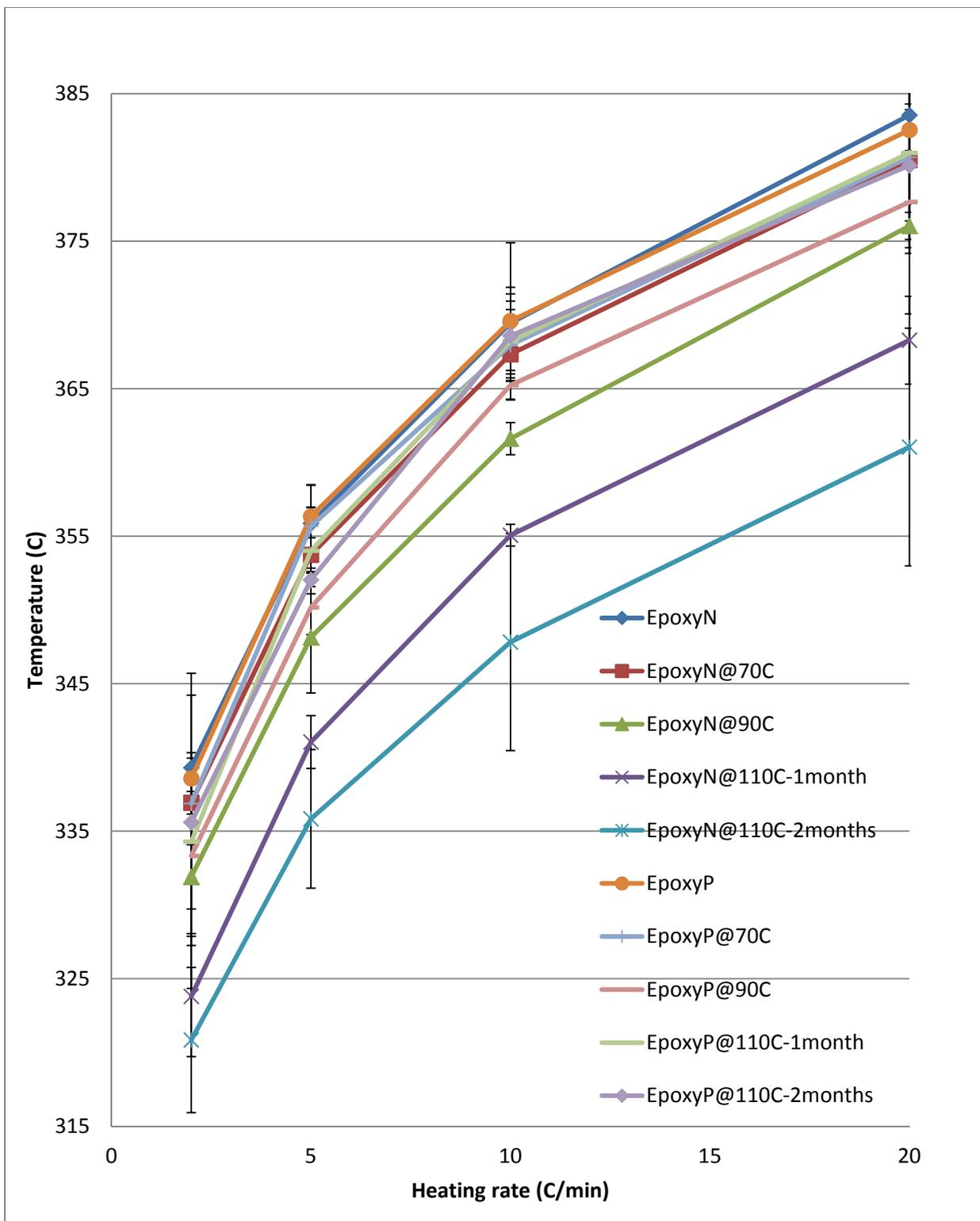
Figure 3: Averaged TGA data for epoxy materials at 10% weight loss. Means and 95% confidence intervals are plotted for three independent TGA measurements.
