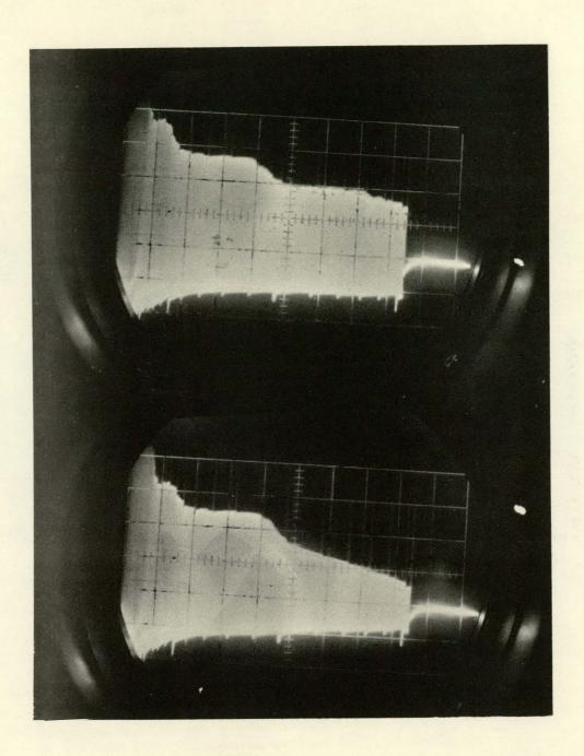
Fig. 2. (a) Top Frame. Bevatron beam intensity versus time as seen by the south sum induction electrodes; 10<sup>10</sup> protons per cm vertical, 200 msec per cm horizontal, filamentary target removed.
