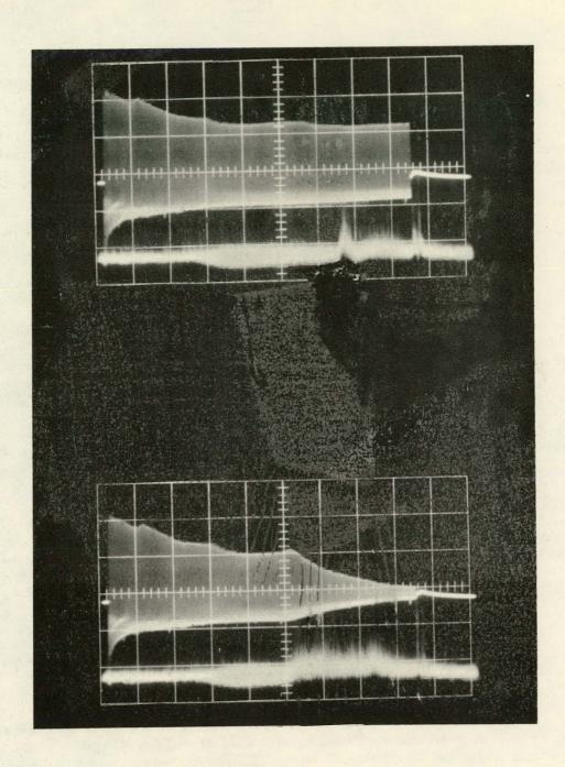
Fig. 4. (a) Top Frame, Top Trace: Bevatron primary-beam intensity versus time as seen by the south sum induction electrode; 10 10 protons per cm, vertical, 200 milliseconds per cm horizontal 100-micron filamentary target removed. Bottom Trace: Ungated scintillation-counter output.
