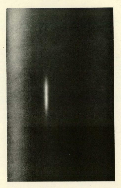
Fig. 1. Radioautograph of an activated 10-micron nylon fibre that was used to produce 1875-millisecond secondary-particle beam with an energy spread from 10 to 6300 Mev. The fibre was placed at a radius of 600 inches in the accelerator aperture.
