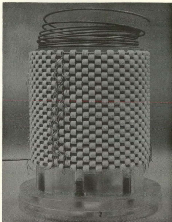
FIGURE 3. Alumina Beads and Lucite Model Used for Fabricating BS-9 Gauge Kanthal Furnace.
