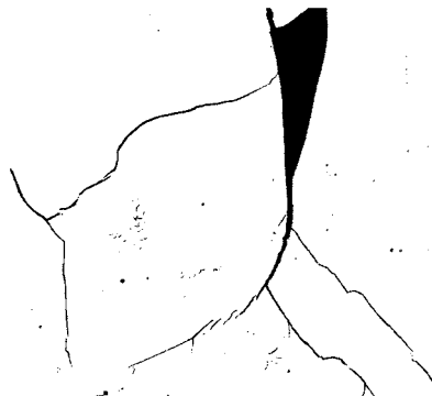
FIGURE 5.7. Tungsten Inclusions in Single Crystal UO_2 Showing Deposition at Capsule Wall. (Unetched)
