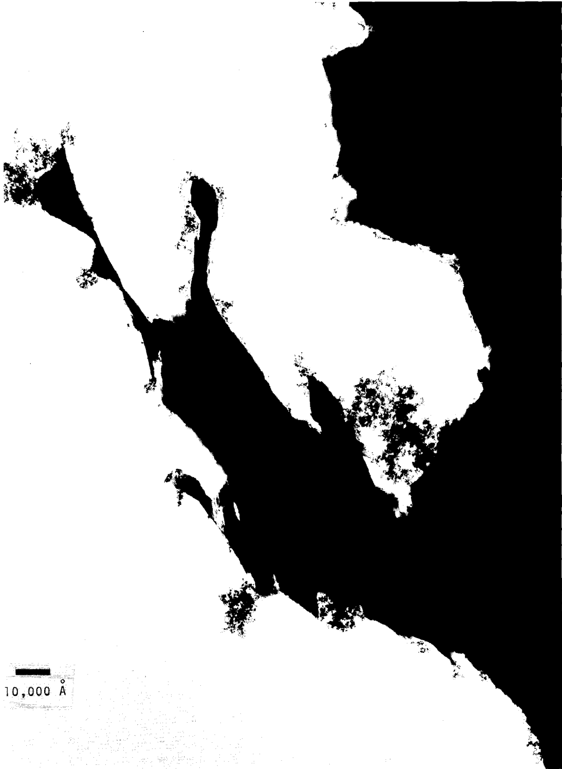
FIGURE 3.1. Lace Network Impurity Areas in AGOT-LS Graphite Exposed to View by Removal of Graphite at Low Temperature with Glowing Microwave-Excited Oxygen and Followed by Thermal Treatment at 700 °C
