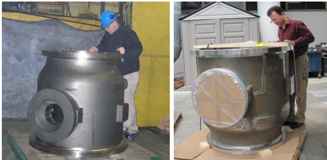
Fig. 3. CF8C-Plus casting of turbine housing at foundry and upon delivery to Solar Turbines.
