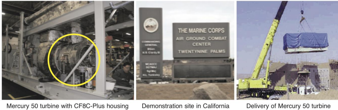
Fig. 4. Update on the Solar Turbines demonstration at a CHP project in California. The CF8C-Plus housing is circled in the picture on the left.
