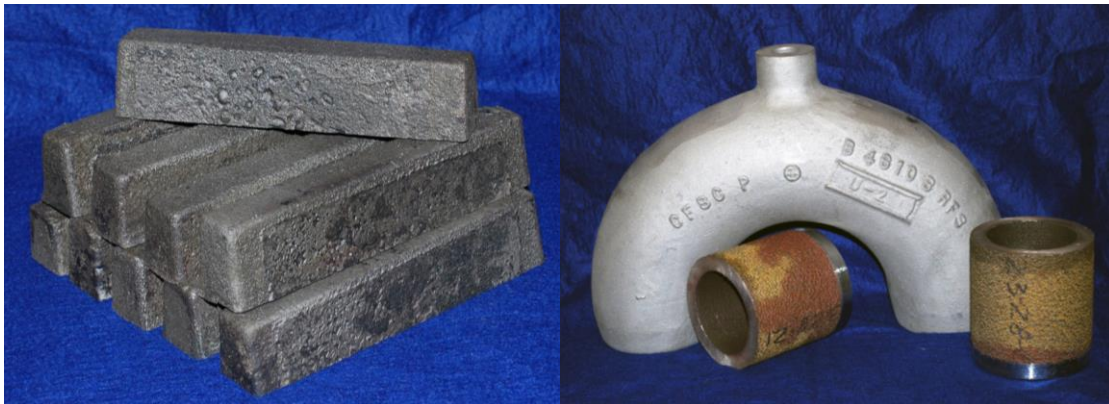
Fig. 5. Keel bars and tube sections from the two commercial orders of CF8C-Plus received in February 2010.
