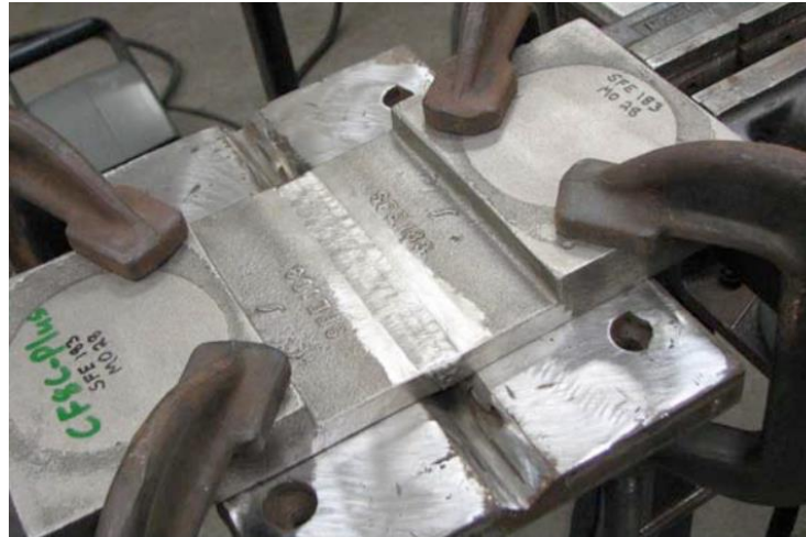
Fig. 8. Gas tungsten arc weld made between two CF8C-Plus plates.
