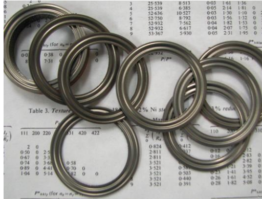
Fig. 19. Stamped bellows segments made from AFA foil.
