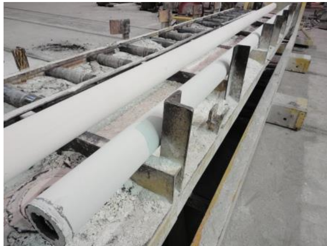
Fig. 8. Cast AFA tube made at Duraloy Technologies.
