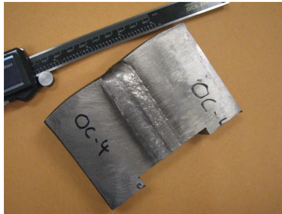
Fig. 17. Welded 10mm OC4 plate being machined into creep specimens.
