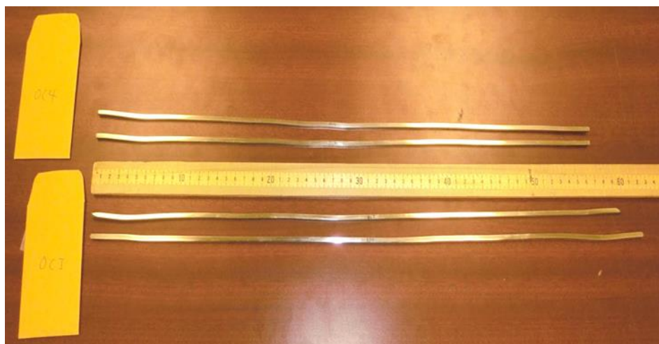
Fig. 37. OC-4 and OC-I rods manufactured by ORNL for gradient metal dusting condition evaluation.
