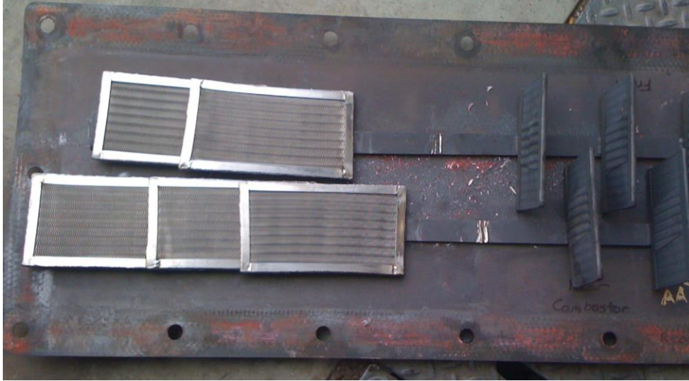
Fig. 7. Panels of folded AFA OC-4 foil to be welded into Mercury 50 turbine by Solar Turbines, Inc.
