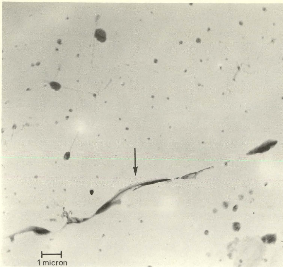
FIGURE 16. Complex Precipitation in Center of Fusion Zone of Weld. Note Long Stringer in Columnar-Grain Boundary (arrow).
