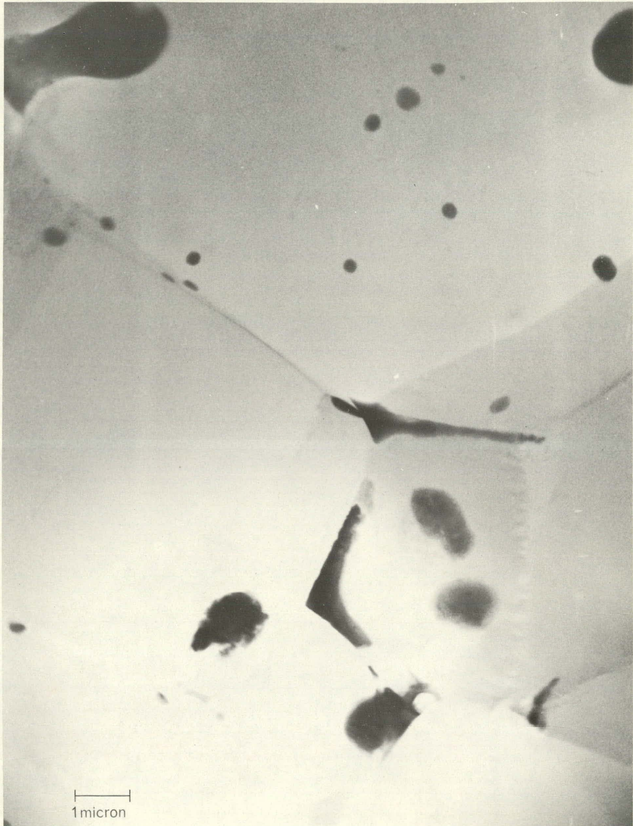
FIGURE 12. Extensive Aluminum-Rich Precipitation along Grain Boundaries in the Vicinity of Intergranular Cracks in the Heat-Affected Zone.
