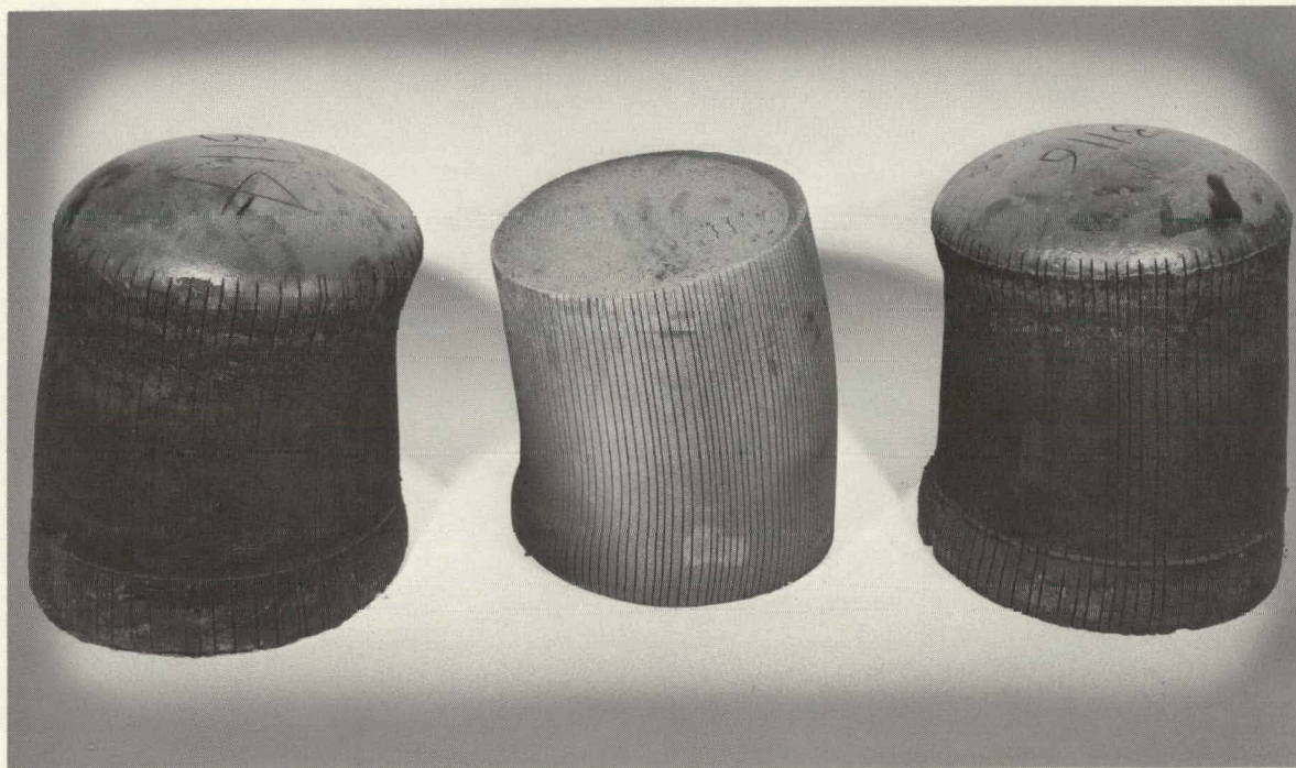
Figure 6. CANTED AND SLUMPED BILLETS.
